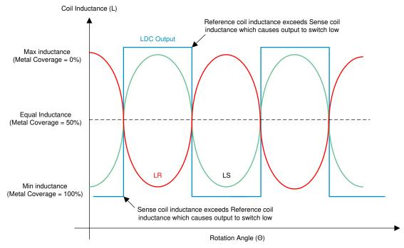
Figure 7-3. Angular Position vs Coil Inductance
