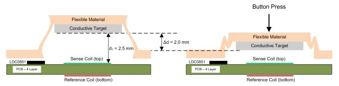
Figure 7-4. Coarse Position Sensing Side View
