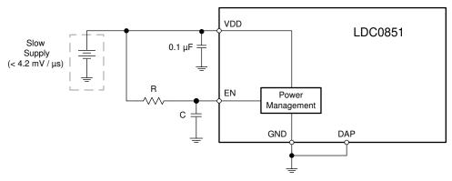
Figure 7-9. Supply Connections for Slow Ramp Rate
