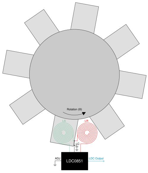
Figure 7-2. Gear Tooth Functional Diagram
