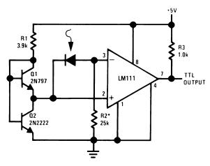
\*R2 sets the comparison level. At comparison, the photodiode has less than 5 mV across it, decreasing leakages by an order of magnitude.
