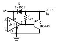
Figure 41. Comparator and Solenoid Driver
