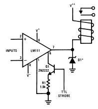
\*Absorbs inductive kickback of relay and protects IC from severe voltage transients on  $V^{++}$  line. **Note:** Do Not Ground Strobe Pin.
