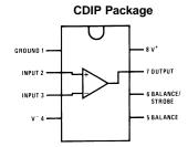
Figure 2. Top View Package Number NAB008A
