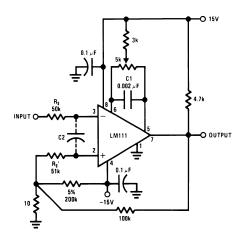
Figure 24. Positive Feedback with High Source Resistance
