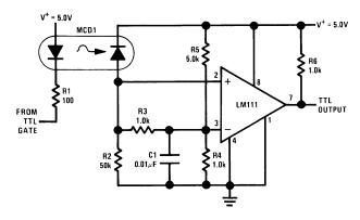
Figure 29. Digital Transmission Isolator
