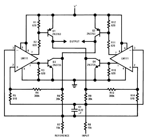
Figure 49. Switching Power Amplifier
