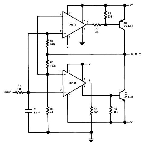
Figure 48. Switching Power Amplifier
