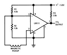
Figure 28. Detector for Magnetic Transducer
