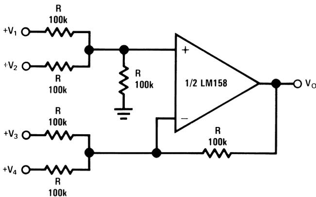
Where:  $V_O = V_1 + V_2 - V_3 - V_4$
