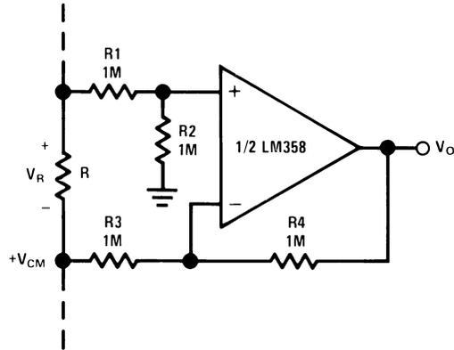
Figure 34. Ground Referencing a Differential Input Signal
