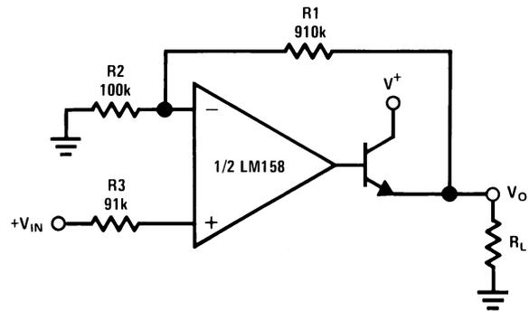
$V_O = 0$  V<sub>DC</sub> for  $V_{IN} = 0$  V<sub>DC</sub>
