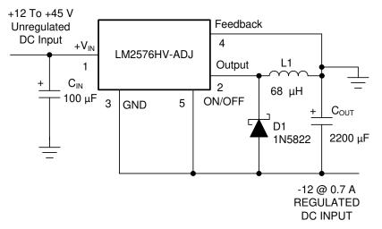
Figure 8-1. Inverting Buck-Boost Develops -12 V
