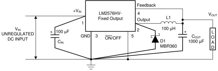
$C_{IN}$  — 100-µF, 75-V, Aluminum Electrolytic  $C_{OUT}$  — 1000-µF, 25-V, Aluminum Electrolytic  $D_1$  — Schottky, MBR360  $L_1$  — 100 µH, Pulse Eng. PE-92108  $R_1$  — 2 k, 0.1%  $R_2$  — 6.12 k, 0.1%
