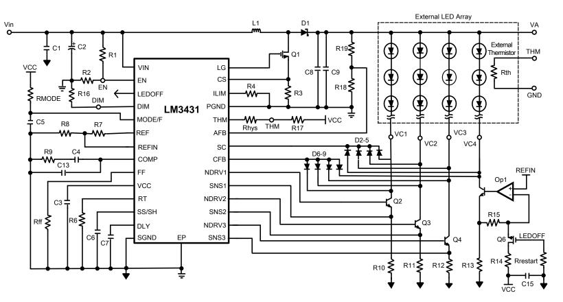
Figure 14. Typical Application Schematic
