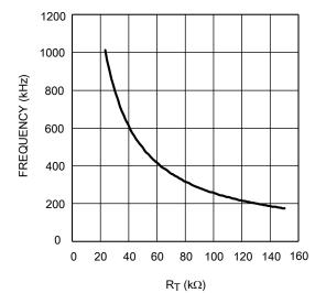
Figure 16. Switching Frequency vs R<sub>T</sub>
