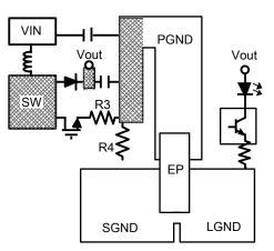
Figure 28. Example PCB Layout
