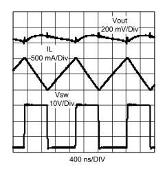
Figure 17. Inductor Current, SW Voltage, and V<sub>OUT</sub>
