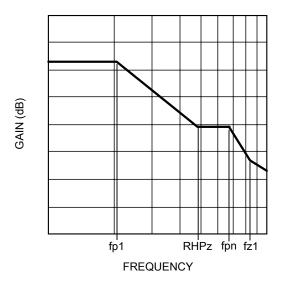
Figure 19. Typical Control-to-Output Bode Plot
