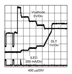
Figure 26. LED String Short Fault and UVP Detection
