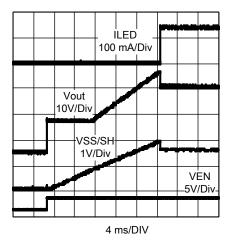
Figure 15. Typical Startup Waveforms (From power-on, DIM = high)
