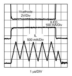
Figure 18. Inductor Current During Dimming
