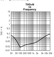
FREQUENCY (Hz) Figure 11.  $V_{DD}$  = 3V; LHP, RHP; P<sub>O</sub> = 10mW; R<sub>L</sub> = 32 $\Omega$ ; Mode 9; 0dB Gain
