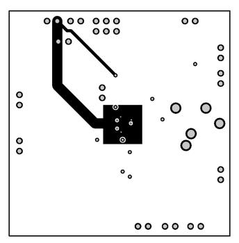
Figure 59. Recommended DSBGA PCB Layout: Inner Layer 2
