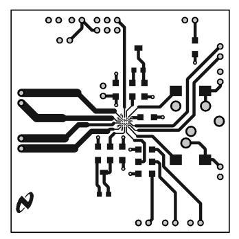
Figure 57. Recommended DSBGA PCB Layout: Top Layer
