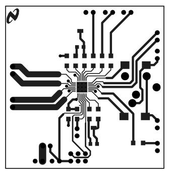
Figure 62. Recommended UQFN PCB Layout: Top Layer
