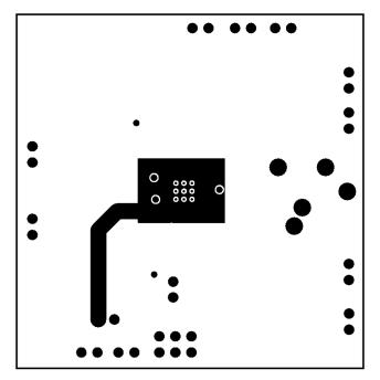
Figure 63. Recommended UQFN PCB Layout: Mid Layer
