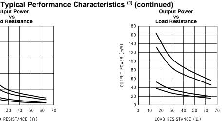
$\begin{array}{l} \mbox{LOAD RESISTANCE ($\Omega$)} \\ \mbox{Figure 47. LHP, RHP; $R_L$ = 32$$\Omega$;} \\ \mbox{Top-V}_{DD} = 5$V, 10\% THD+N; Topmid-V}_{DD} = 5$V, 1% THD+N; \\ \mbox{Botmid-V}_{DD} = 3$V, 10\% THD+N; Bot-V}_{DD} = 3$V, 1% THD+N \\ \end{array}$
