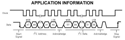
Figure 53. I<sup>2</sup>C Bus Format
