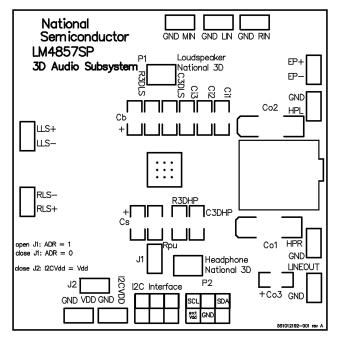
Figure 61. Recommended UQFN PCB Layout: Top Over Layer
