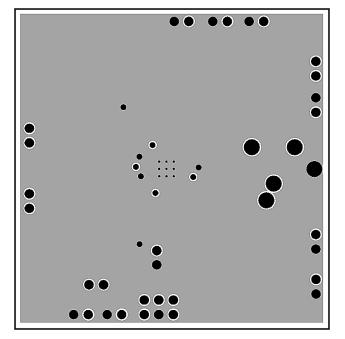
Figure 64. Recommended UQFN PCB Layout: Bottom Layer
