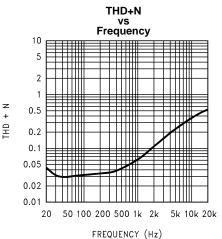
Figure 13.  $V_{DD} = 3V$ ; EP; P<sub>0</sub> = 10mW; R<sub>L</sub> = 32 $\Omega$ ; Mode 1; 0dB Gain, CD4 = 0
