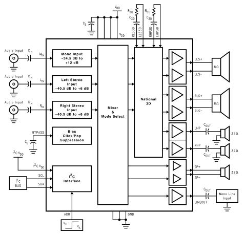
Figure 1. Typical Audio Amplifier Application Circuit
