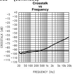
Figure 35.  $V_{DD}$  = 3V; LHP, RHP;  $P_O$  = 10mW;  $R_L$  = 32 $\Omega$ ; Mode 9; 0db Gain; 3D off Top-Left to Right; Bot- Right to Left
