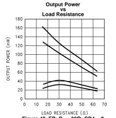
Figure 48. EP;  $R_L = 32\Omega$ ; CD4 = 0 Top-V<sub>DD</sub> = 5V, 10% THD+N; Topmid-V<sub>DD</sub> = 5V, 1% THD+N; Botmid-V<sub>DD</sub> = 3V, 10% THD+N; Bot-V<sub>DD</sub> = 3V, 1% THD+N
