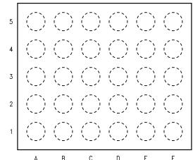
Figure 2. 30 Bump DSBGA Package – Top View (Bump-side down) See Package Number YZR0030
