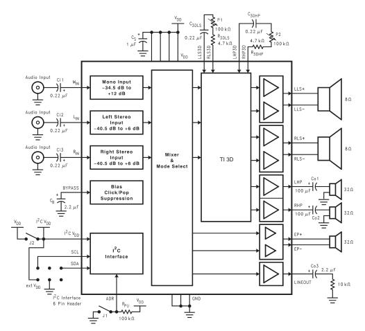
Figure 55. Reference Design Board Schematic
