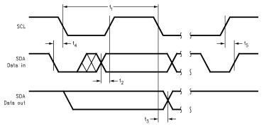
Figure 54. I<sup>2</sup>C Timing Diagram
