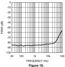
PSRR vs Frequency  $V_{DD} = 3V$ ,  $R_L = 8\Omega$ , Input  $10\Omega$  Terminated
