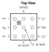
Figure 1. VSSOP Package See Package Number DGS0010A
