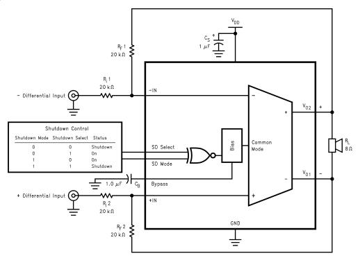
Figure 4. Typical Audio Amplifier Application Circuit
