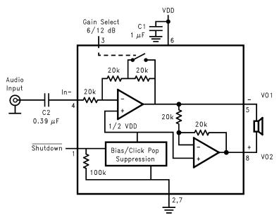
Figure 1. Typical Audio Amplifier Application Circuit
