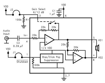
Figure 26. REFERENCE DESIGN BOARD SCHEMATIC
