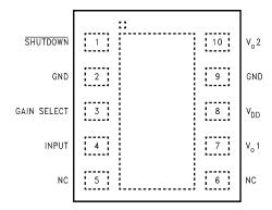
Figure 2. VSSOP Package (Top View) See Package Number DGK
