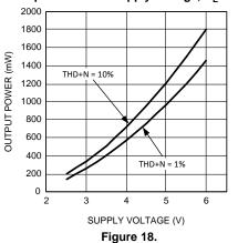
Output Power vs Supply Voltage,  $R_L = 32\Omega$
