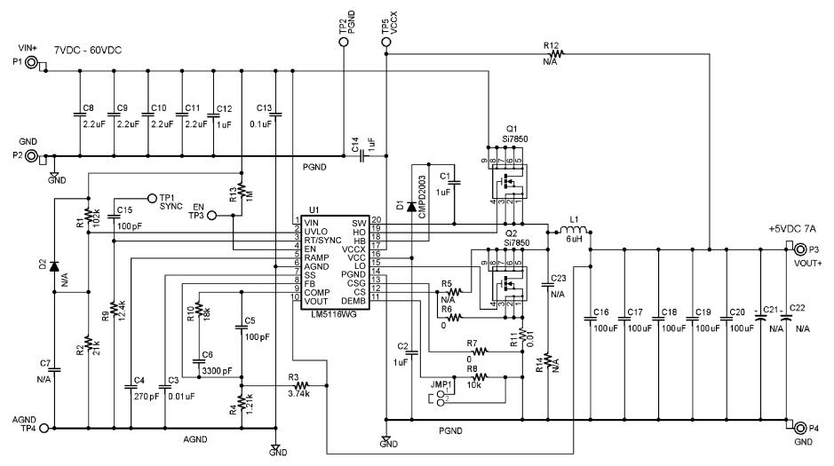
Figure 41. 5V 7A Typical Application Schematic
