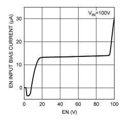
Figure 30. EN Bias Current vs Voltage
