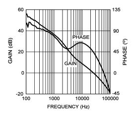
Figure 38. Overall Voltage Loop Gain and Phase
