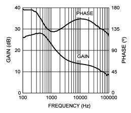
Figure 37. Error Amplifier Gain and Phase
