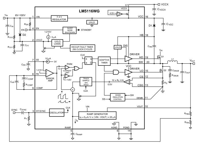
**Block Diagram and Typical Application Circuit**
