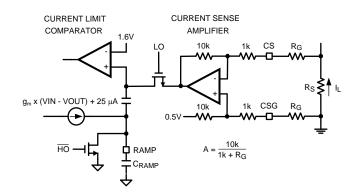
Figure 33. Current Limit and Ramp Circuit
