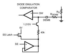
Figure 34. Diode Emulation Control
