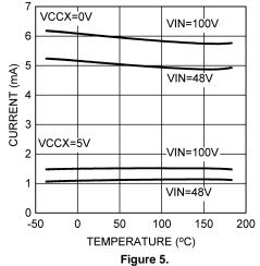
RAMP Current vs Temperature
