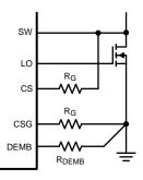
Figure 32. R<sub>DS(ON)</sub> Current Sensing without Diode Emulation
