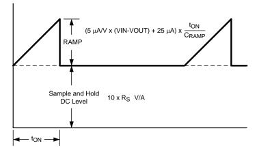
Figure 31. Composition of Current Sense Signal
