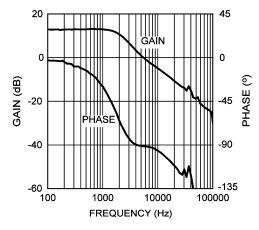
Figure 36. Modulator Gain and Phase
