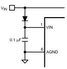
Figure 28. Input Blocking Diode for VCCX > VIN
