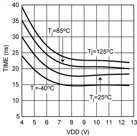
Figure 11. OUT Turnon Propagation Delay vs VDD
