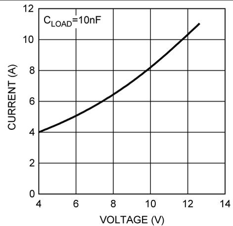
**Figure 6. OUT Peak Sink Current vs VDD Voltage**
