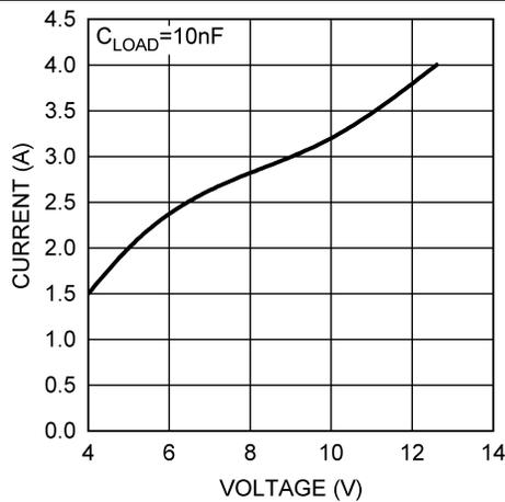
**Figure 5. OUT Peak Source Current vs VDD Voltage**
