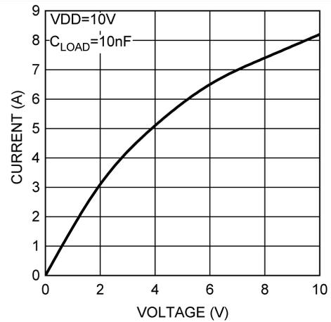
**Figure 4. OUT Sink Current vs OUT Voltage**
