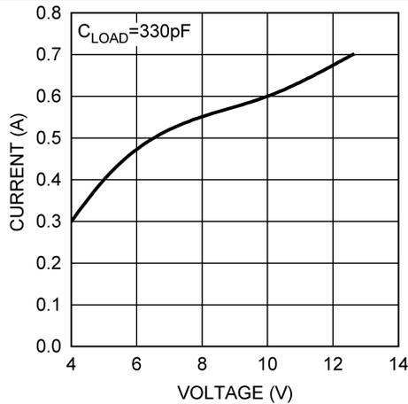
Figure 9. PILOT Peak Source Current vs VDD Voltage
