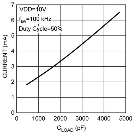
Figure 15. Supply Current vs OUT Capacitive Load
