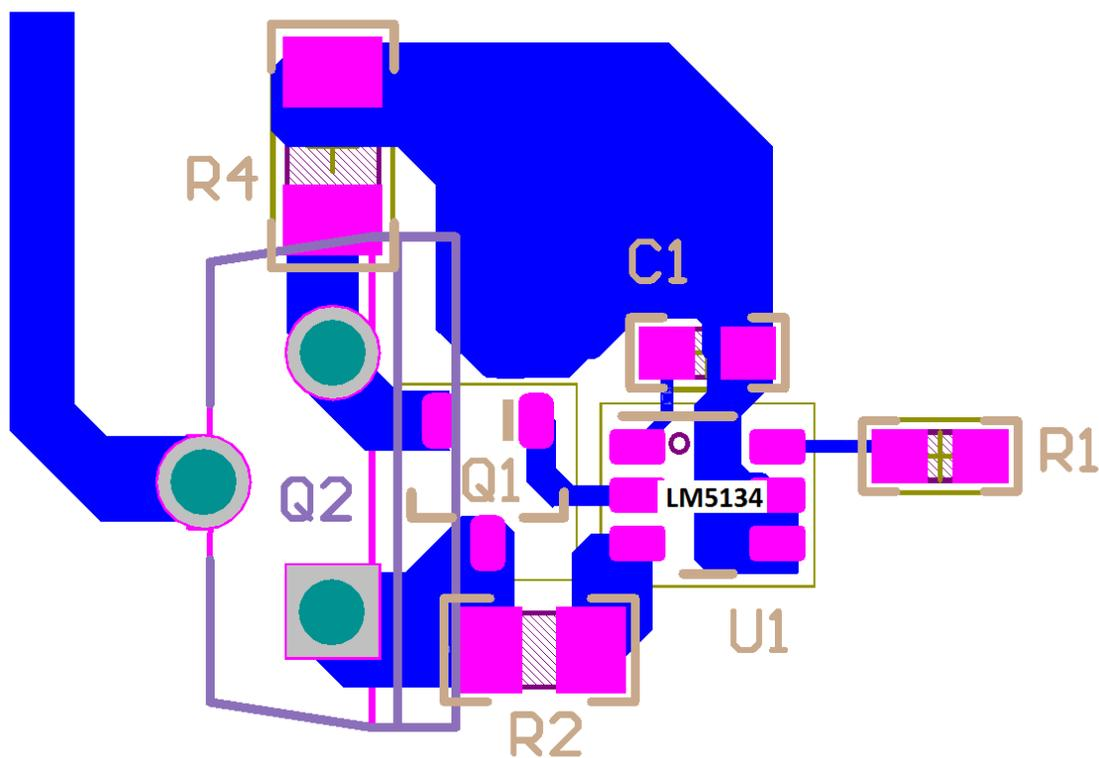
Figure 27. LM5134 Layout Example
