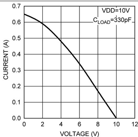
**Figure 7. PILOT Source Current vs PILOT Voltage**
