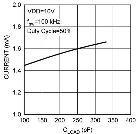
Figure 16. Supply Current vs PILOT Capacitive Load
