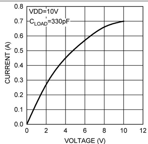
**Figure 8. PILOT Sink Current vs PILOT Voltage**
