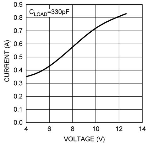
Figure 10. PILOT Peak Sink Current vs VDD Voltage
