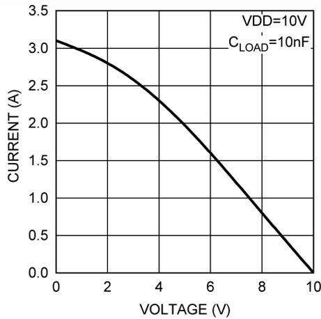
**Figure 3. OUT Source Current vs OUT Voltage**
