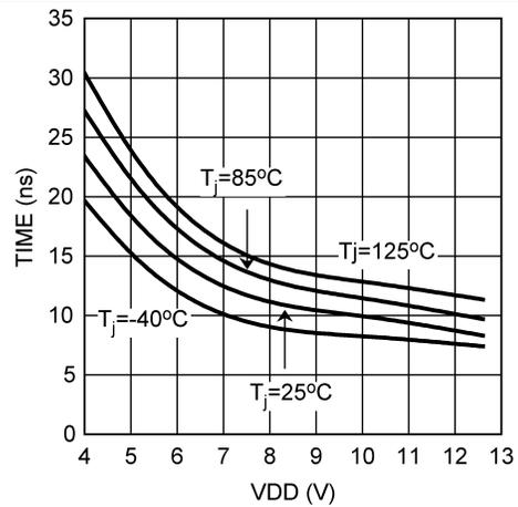
Figure 12. OUT Turnoff Propagation Delay vs VDD
