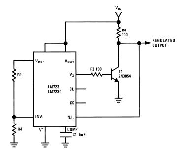
Regulated Output Voltage Line Regulation ( $\Delta V_{IN} = 10V$ ) Load Regulation ( $\Delta I_L = 100$  mA) +5V
