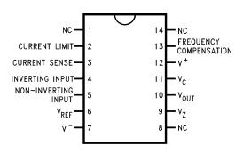
Figure 1. Top View CDIP Package or PDIP Package See Package J or NFF0014A
