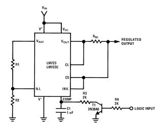
Note: Current limit transistor may be used for shutdown if current limiting is not required.
