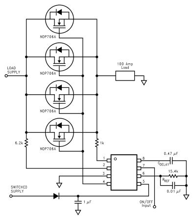
Figure 19. Driving Multiple MOSFETs
