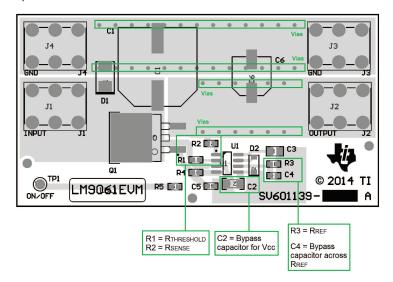
Figure 26. LM9061EVM Layout Example (Top)
