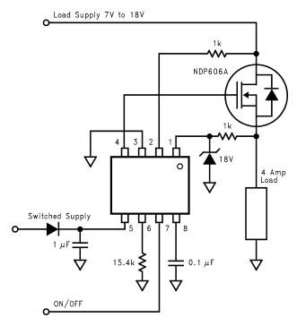
Figure 16. Adding Overvoltage Protection
