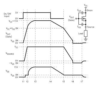
Figure 13. Turnon and Turnoff Waveforms
