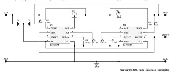
Figure 24. Bidirectional Switch Including Reverse OCP
