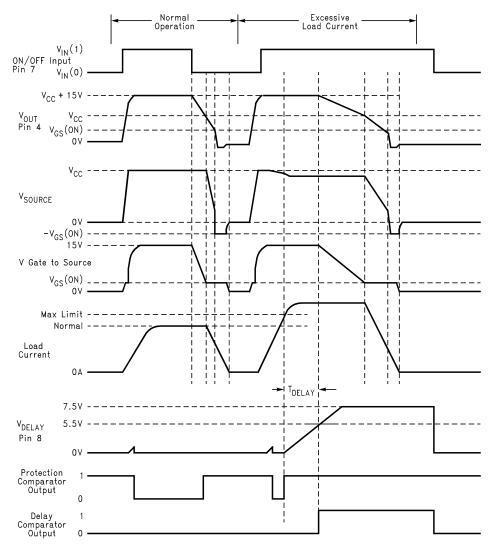
Figure 1. Typical Operating Waveforms
