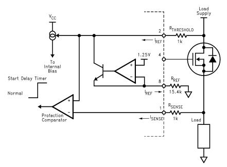
Figure 14. Protection Comparator Biasing
