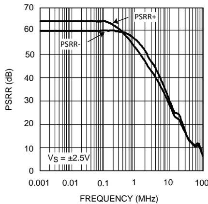
Figure 21. PSRR vs. Frequency
