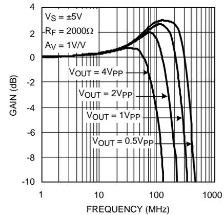
Figure 4. Frequency Response vs.  $V_{OUT}$ ,  $A_V = 1$
