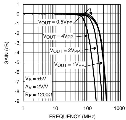
Figure 2. Frequency Response vs.  $V_{OUT}$ ,  $A_V = 2$
