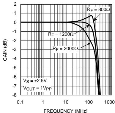
**Figure 31. Frequency Response vs.  $R_F$**
