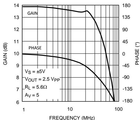
**Figure 38. Composite Amplifier Frequency Response**
