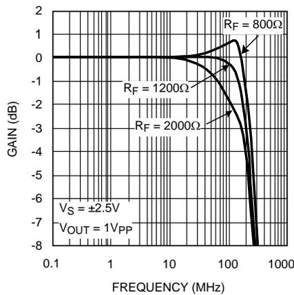
Figure 9. Frequency Response vs.  $R_F$
