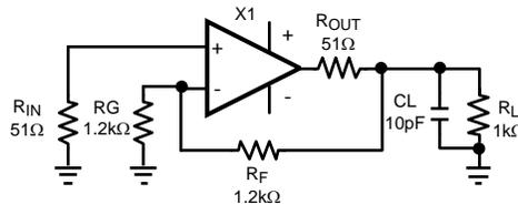
Figure 36. Series Output Resistor Inside Feedback Loop
