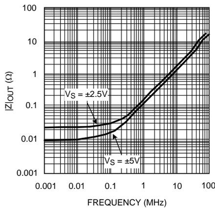
Figure 23. Closed Loop Output Resistance
