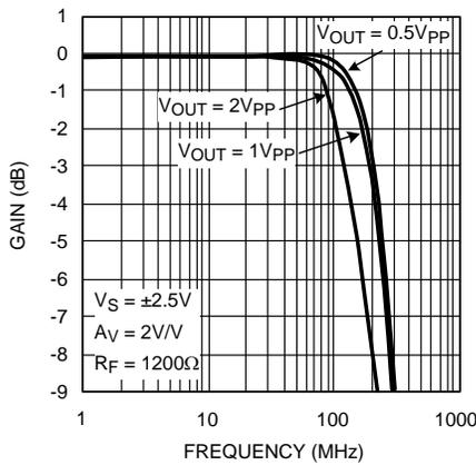
Figure 1. Frequency Response vs.  $V_{OUT}$ ,  $A_V = 2$
