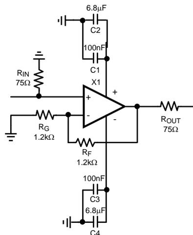
**Figure 34. Typical Application with Suggested Supply Bypassing**
