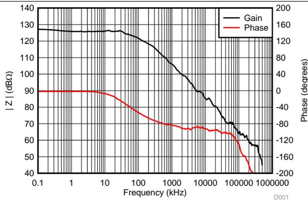
Figure 11. Open Loop Gain & Phase
