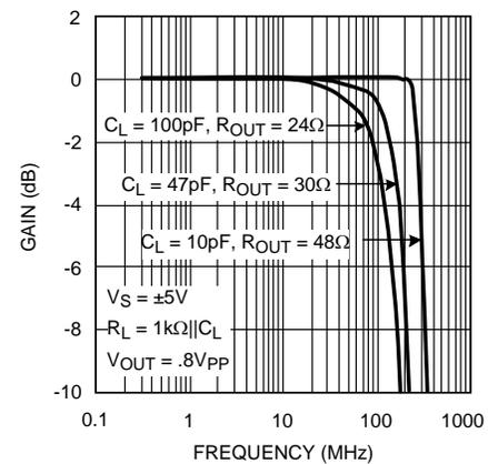
Figure 18. Frequency Response vs.  $C_L$
