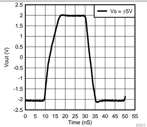
Figure 30. Output Large Signal Pulse Response
