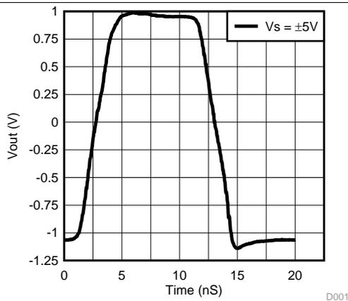
Figure 29. Output Small Signal Pulse Response
