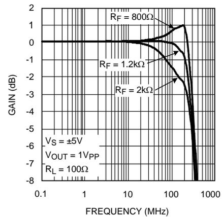
Figure 10. Frequency Response vs.  $R_F$
