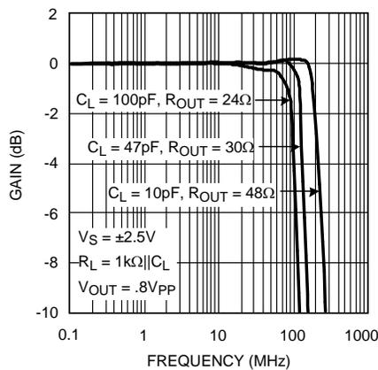
Figure 17. Frequency Response vs.  $C_L$
