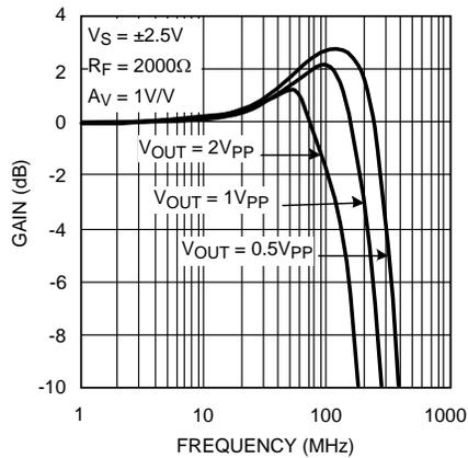
Figure 3. Frequency Response vs.  $V_{OUT}$ ,  $A_V = 1$
