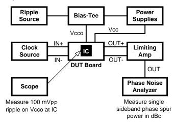
Figure 39. PSRR Test Setup
