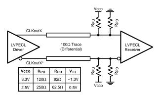
Figure 32. Differential LVPECL Operation, DC Coupling, Thevenin Equivalent
