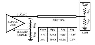
Figure 37. Single-Ended LVPECL Operation, DC Coupling, Thevenin Equivalent
