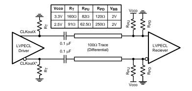
Figure 35. Differential LVPECL Operation, AC Coupling, Thevenin Equivalent
