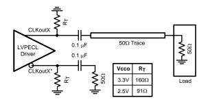
Figure 38. Single-Ended LVPECL Operation, AC Coupling
