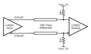
Figure 31. Differential LVPECL Operation, DC Coupling
