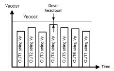
Figure 17. Boost Adaptive Control Principle with PSPWM
