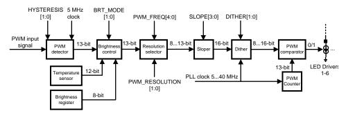
Figure 13. PWM Calculation Data Flow
