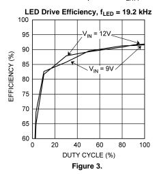
LED Drive Efficiency, f<sub>LED</sub> = 19.2 kHz, External FET
