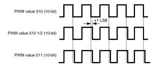
Figure 16. Example of the Dithering, 1-bit dither, 10-bit resolution
