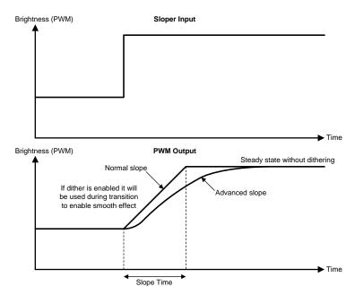
Figure 15. Sloper Operation
