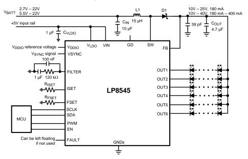
**Note:** Separate 5V rail to  $V_{LDO}$  can be also used to improve efficiency for applications with higher battery voltage. No power sequencing requirements between  $V_{IN}/V_{LDO}$  and  $V_{BATT}$ .
