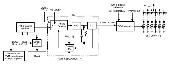
Figure 12. Principle of the Clock Generation
