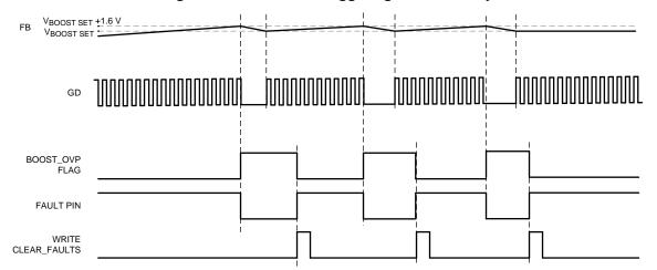
Figure 41. Boost OVP Triggering and Recovery
