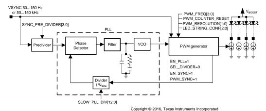
Figure 12. PWM Synchronization With External VSYNC Input
