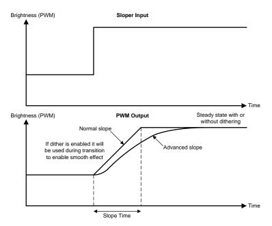
Figure 14. Sloper Operation
