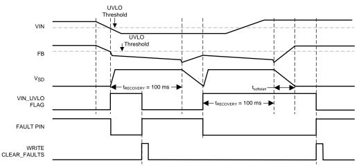
Figure 38. Input UVLO Triggering and Recovery
