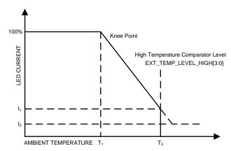
Figure 33. Current Dimming for High Ambient Temperature
