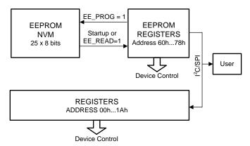
Figure 44. EEPROM and Register Configuration
