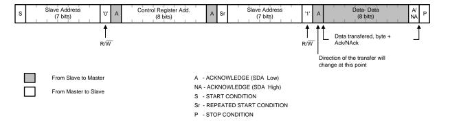
Figure 52. Register Read Format
