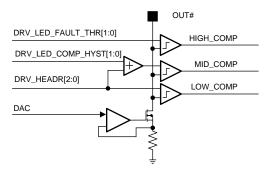
Figure 28. Output Voltage Comparators
