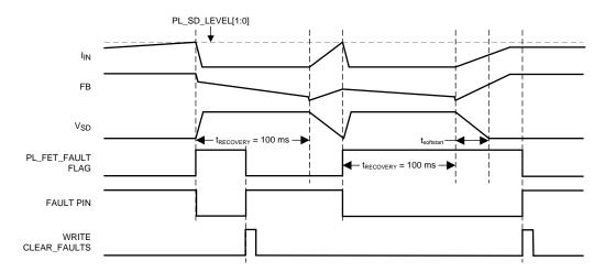
Figure 39. Input OVP Triggering and Recovery
