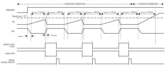
Figure 40. Boost OCP Triggering and Recovery
