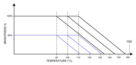
Figure 30. Thermal De-Rating Function Example With 100% and 50% Brightness
