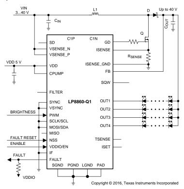
Figure 66. Solution With Minimum External Components
