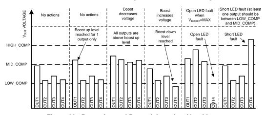
Figure 29. Protection and Boost Adaptation Algorithms
