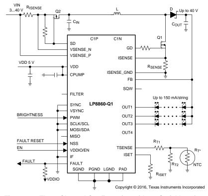
Figure 63. Three-Channel Configuration without Serial Interface
