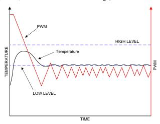
Figure 31. LED Current Limitation With NTC
