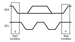
Figure 49. Stop and Start Conditions
