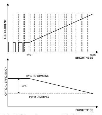
Figure 16. Optical Efficiency Improvement With PWM and Current Dimming
