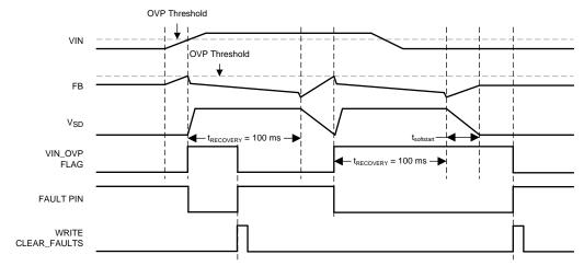
Figure 37. Input OVP Triggering and Recovery
