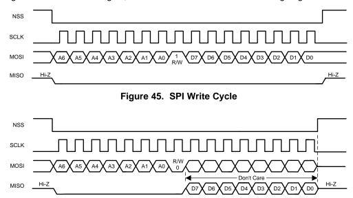
Figure 46. SPI Read Cycle
