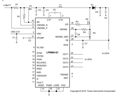
Figure 55. Critical Components for Design
