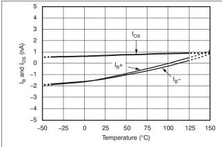
Figure 13. Input Bias and Input Offset Currents vs Temperature
