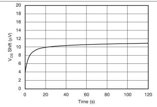
Figure 15. Input Offset Voltage vs Time
