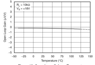
Figure 10. Open-Loop Gain vs Temperature
