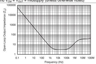
Figure 8. Open-Loop Output Impedance vs Frequency
