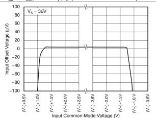
Figure 14. Input Offset Voltage vs Common-Mode Voltage
