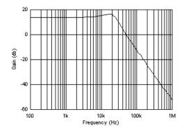
Figure 36. OPAx209 Second-Order, 25-kHz, Chebyshev, Low-Pass Filter
