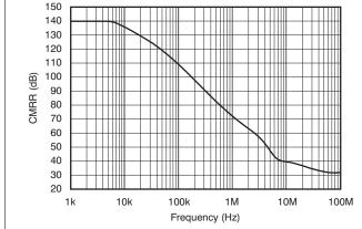
Figure 7. Common-Mode Rejection Ratio vs Frequency
