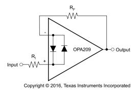
Figure 31. Pulsed Operation
