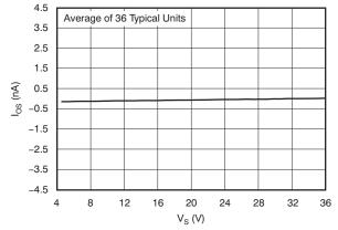
Figure 16. Input Offset Current vs Supply Voltage
