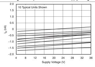
Figure 18. Input Bias Current vs Supply Voltage
