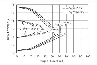
Figure 6-7. OPA365-Q1 Output Voltage vs Output Current
