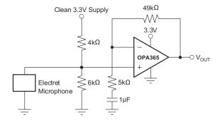
Figure 7-2. Microphone Preamplifier
