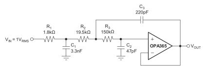
Figure 8-4. Configured as a 3-Pole, 20 kHz, Sallen-Key Filter
