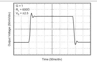
Figure 6-17. Large-Signal Step Response
