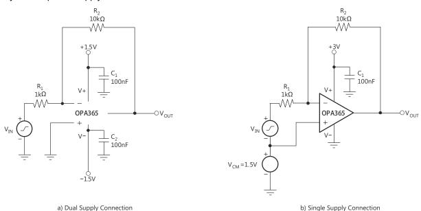
Figure 7-1. Basic Circuit Connections
