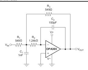
Figure 8-3. Second-Order Butterworth 500-kHz Low-Pass Filter
