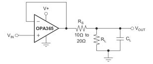
Figure 8-1. Improving Capacitive Load Drive
