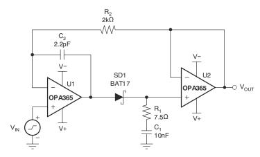
Figure 8-7. Fast Settling Peak Detector Schematic
