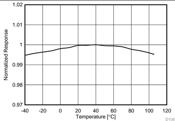
Figure 12. Normalized Response vs Temperature (Grade 2)
