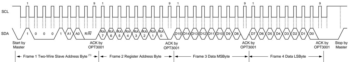
(1) The value of the slave address byte is determined by the setting of the ADDR pin; see Table 1.
