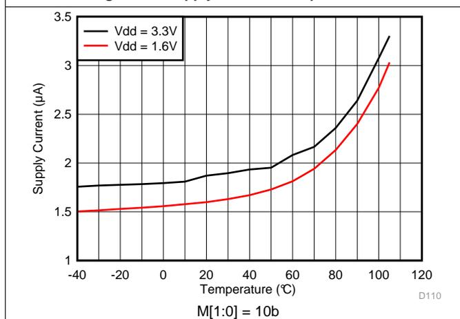
**Figure 18. Supply Current vs Temperature (Grade 2)**
