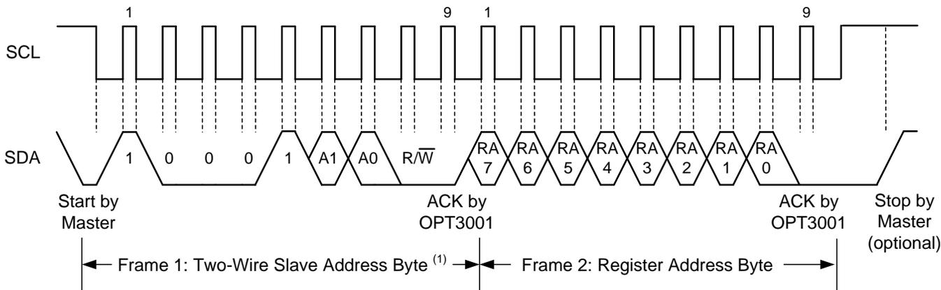
(1) The value of the slave address byte is determined by the ADDR pin setting; see [Table 1](#).
