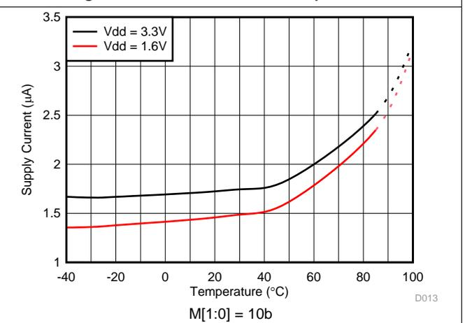
**Figure 19. Supply Current vs Temperature (Grade 3)**
