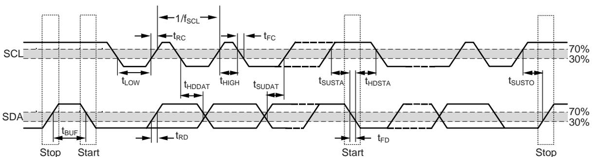
**Figure 1. I<sup>2</sup>C Detailed Timing Diagram**
