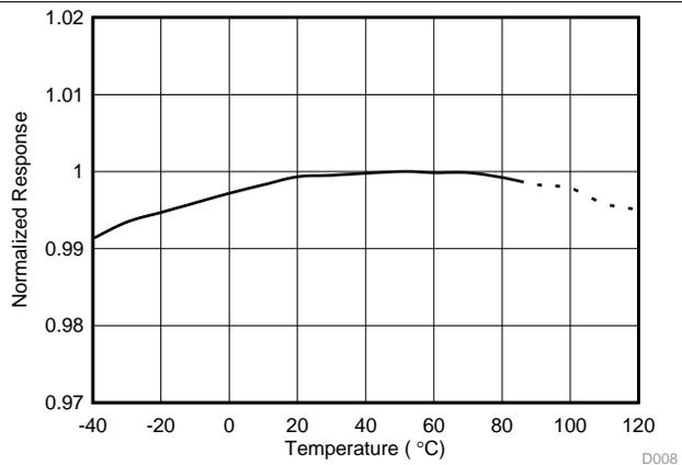
Figure 13. Normalized Response vs Temperature (Grade 3)
