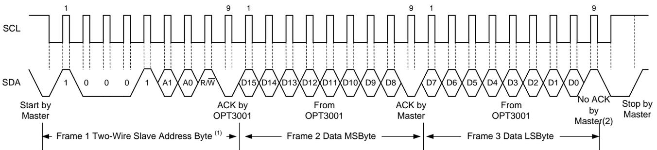
(1) The value of the slave address byte is determined by the ADDR pin setting; see Table 1.
