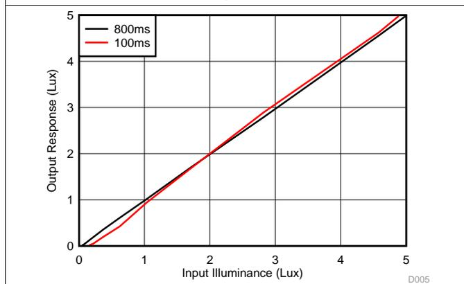
**Figure 6. Output Response vs Input Illuminance: Low Range = 0 lux to 5 lux**
