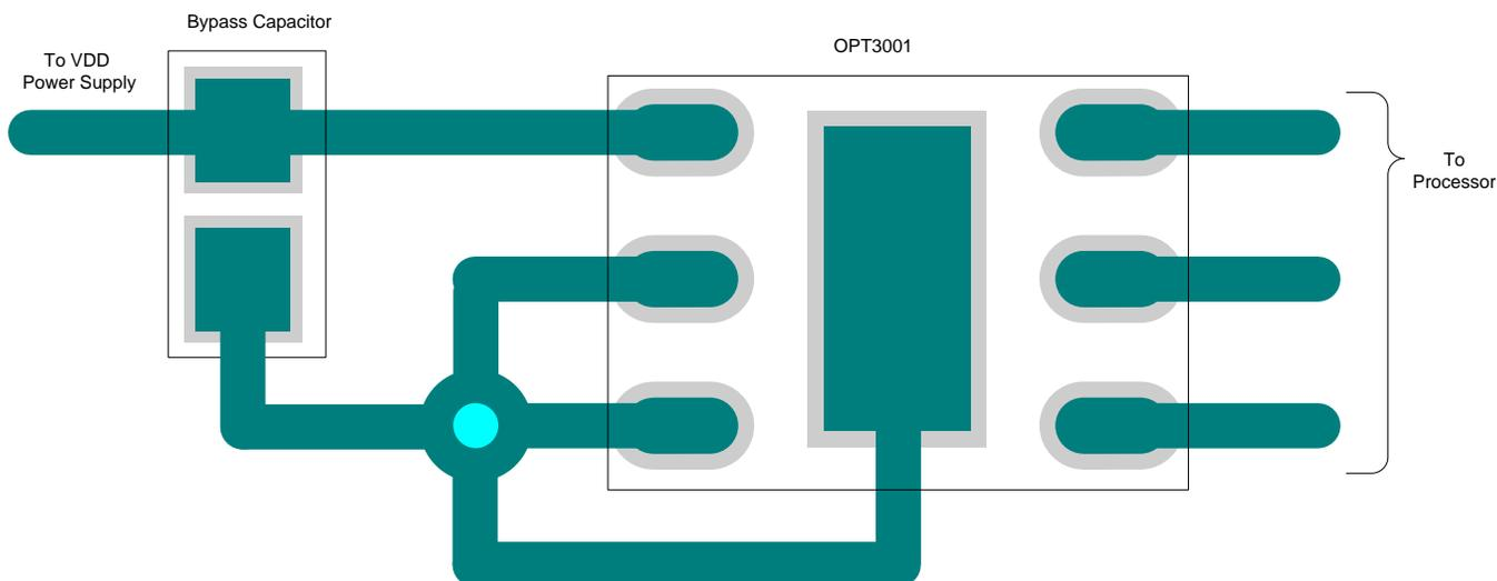
Figure 39. Example PCB Layout With the OPT3001-Q1 Device
