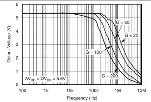
Figure 39. PGA113, PGA117 Output Voltage Swing vs Frequency
