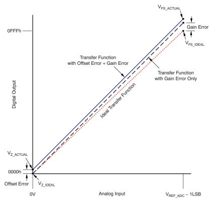
Figure 73. ADC Offset and Gain Error
