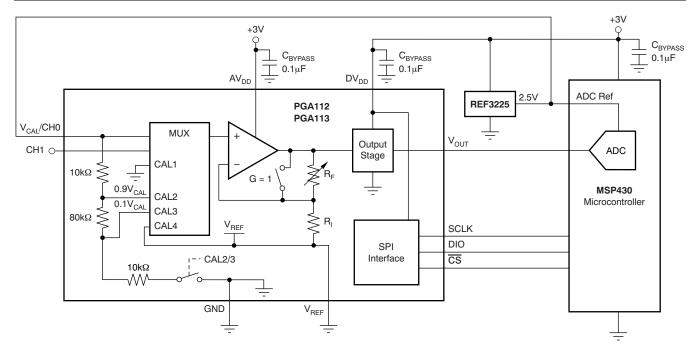
Figure 71. Using CAL Channels With  $V_{REF}$  = Ground
