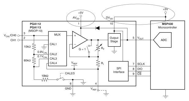
Figure 76. Split Power-Supply Architecture: AV<sub>DD</sub> ≠ Dv<sub>DD</sub>
