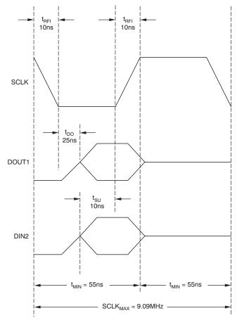
Figure 61. Daisy-Chain Maximum SCLK Frequency
