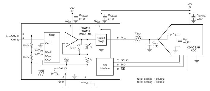
Figure 75. Driving and Interfacing to ADCs
