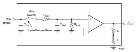
Figure 55. Equivalent Input Circuit
