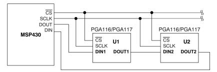
Figure 59. Daisy-Chain Read and Write Configuration
