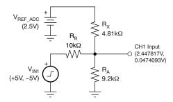
Figure 79. Bipolar to Single-Ended Input Algorithm
