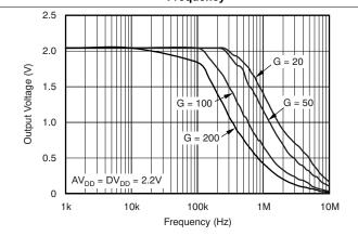
Figure 37. PGA113, PGA117 Output Voltage Swing vs Frequency
