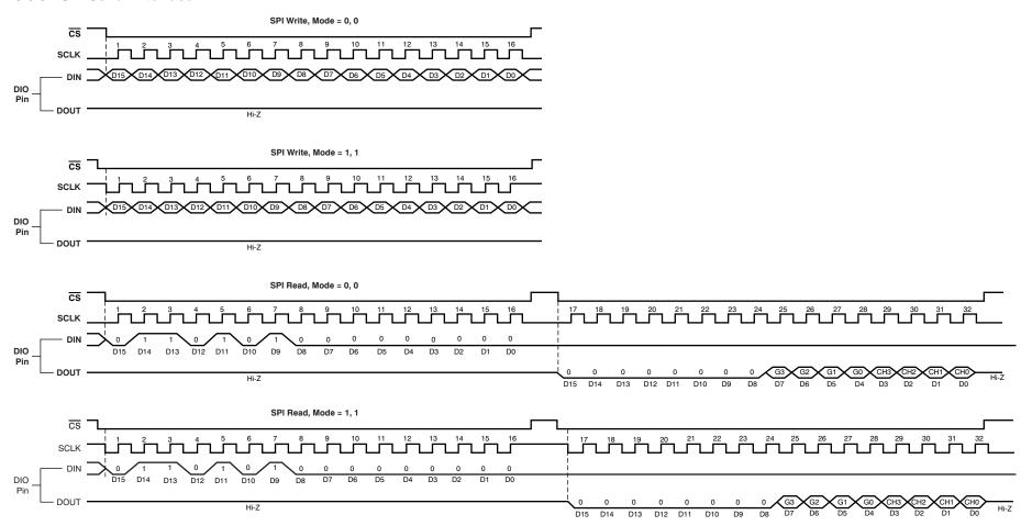
Figure 62. SPI Serial Interface Timing Diagrams
