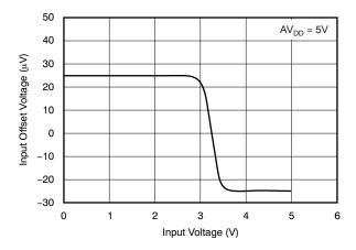
Figure 68. V<sub>OS</sub> Versus Input Voltage—Case 2
