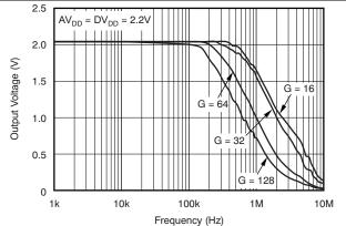
Figure 33. PGA112, PGA116 Output Voltage Swing vs Frequency
