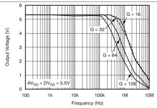
Figure 35. PGA112, PGA116 Output Voltage Swing vs Frequency
