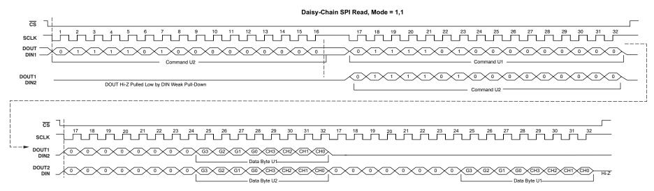
Figure 65. SPI Daisy-Chain Read Timing Diagram (Mode 1,1)
