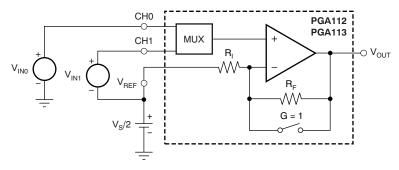
Figure 70. PGA112 and PGA113 Configuration for Positive and Negative Excursions Around Midsupply Virtual Ground
