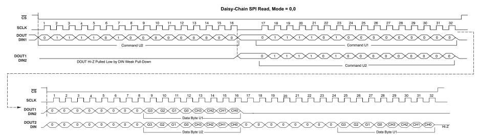
Figure 64. SPI Daisy-Chain Read Timing Diagram (Mode 0,0)
