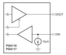
Figure 57. Digital I/O Structure—PGA116 and PGA117
