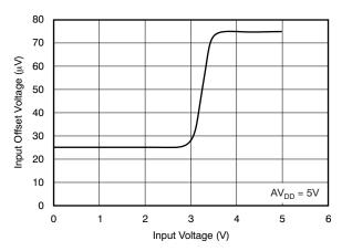
Figure 67. Vos Versus Input Voltage—Case 1
