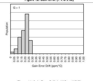
Figure 14. Gain Error Drift (-40°C to 125°C)
