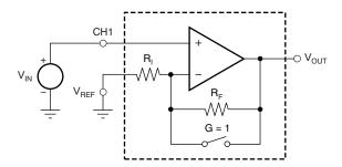
Figure 69. PGA Used as a Gain Block
