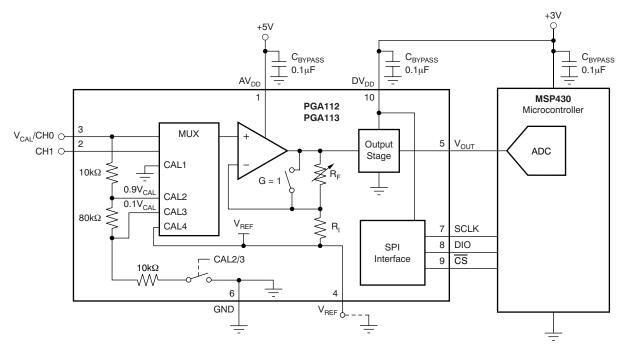
Figure 77. PGA112, PGA113 (VSSOP-10) Typical Application Schematic
