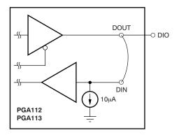
Figure 58. Digital I/O Structure—PGA112 and PGA113
