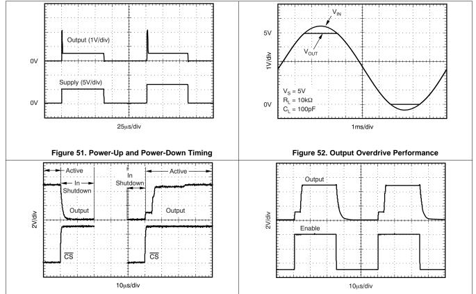
Figure 54. PGA116, PGA117 Hardware Shutdown Mode
