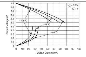
Figure 31. Output Voltage vs Output Current
