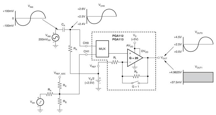
Figure 81. General-Purpose Input Scaling
