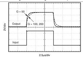
Figure 49. Large-Signal Pulse Response
