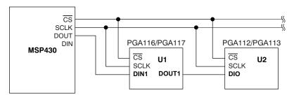
Figure 60. Daisy-Chain Write-Only Configuration
