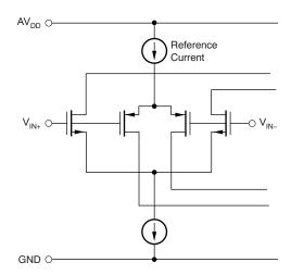
Figure 66. PGA Rail-To-Rail Input Stage
