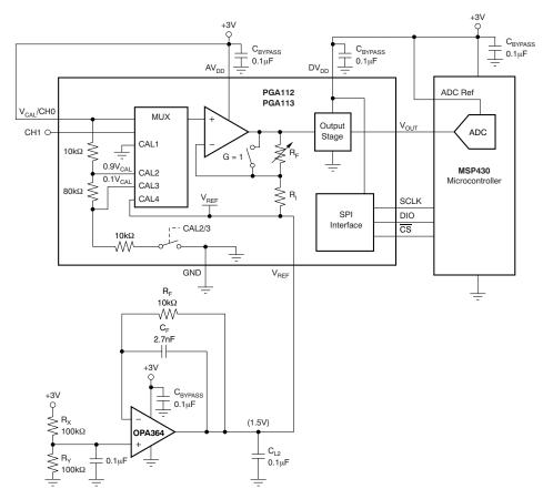
Figure 72. Using CAL Channels With  $V_{REF} = AV_{DD}/2$
