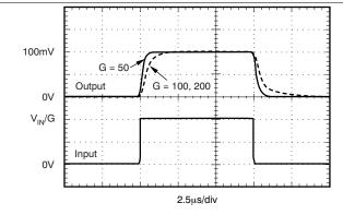
Figure 47. Small-Signal Pulse Response
