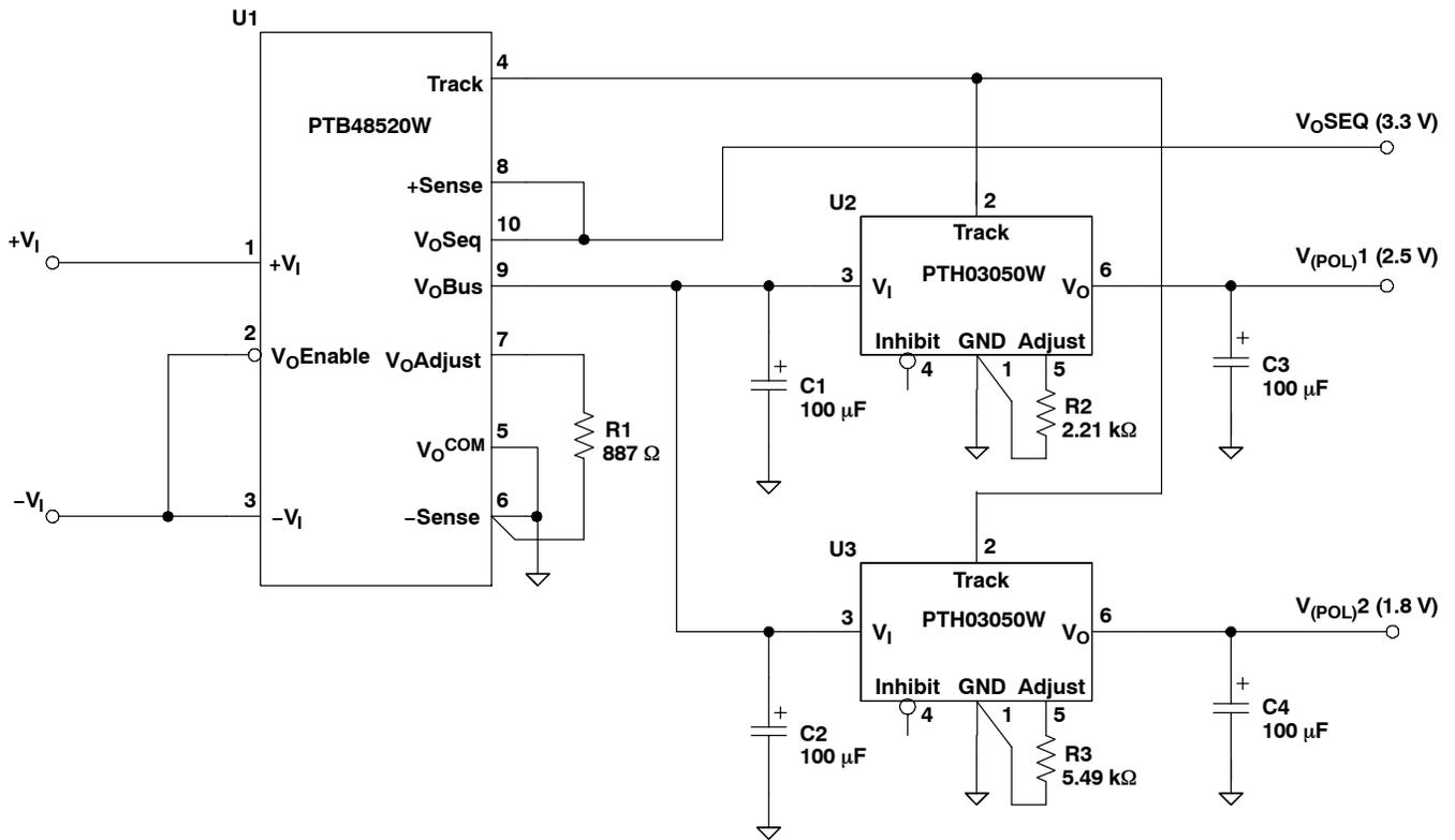
**Figure 10. Power-Up Sequencing With Non-Isolated POL Modules**
