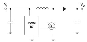
Figure 16. Typical Boost Converter Topology
