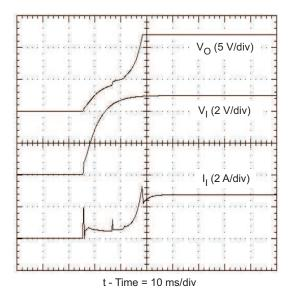
Figure 15. Power-Up Waveforms
