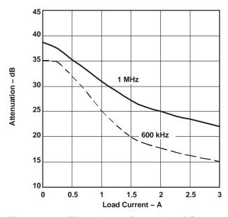
Figure 19. π-Filter Attenuation vs. Load Current
