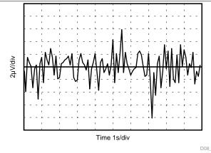
Figure 19. Load Regulation Sinking
