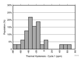
Figure 25. Thermal Hysteresis Distribution (V<sub>RFF</sub>)
