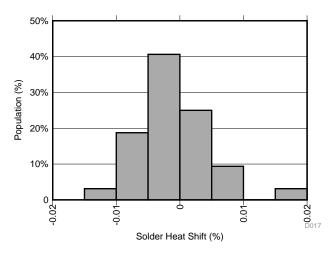
Figure 23. Solder Heat Shift Distribution, V<sub>RFF</sub> (%)
