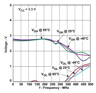
Figure 2. Maximum Switching Frequency  $V_{CC}$ = 3.3 V
