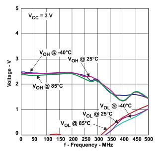
Figure 1. Maximum Switching Frequency V<sub>CC</sub>= 3.0 V
