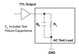
Figure 4. TTL Output AC Test Loading Condition
