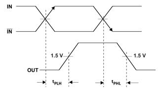
Figure 5. Output Propagation Delay
