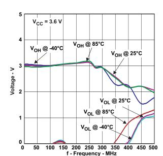
Figure 3. Maximum Switching Frequency V<sub>CC</sub>= 3.6 V
