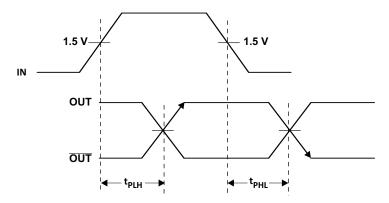
Figure 2. Output Propagation Delay
