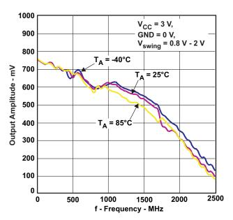
Figure 5. Output Amplitude versus Frequency
