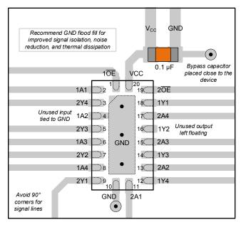
Figure 7-1. Example Layout for the SN74AC241
