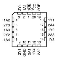
Figure 3-1. SN54ACT241 J or W Package SN74ACT241 DB, DW, N, NS, or PW Package (Top View)
