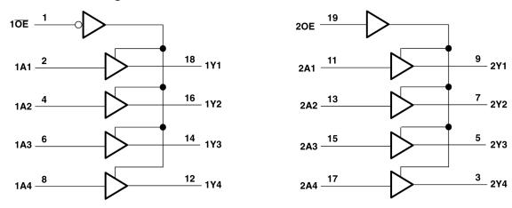
Figure 6-1. Logic Diagram (Positive Logic)
