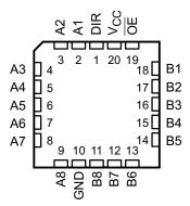
Figure 4-1. SN54ACT245 J or W Package; SN74ACT245 DB, DGS, DW, N, NS, or PW Package Top View
