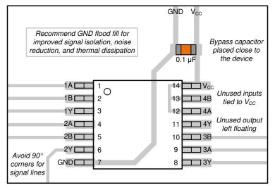
Figure 9-1. Example Layout for the SN74AHC373
