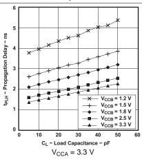
Figure 9. Typical Propagation Delay  $t_{\rm PLH}$  (A to B) vs Load Capacitance
