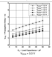
Figure 10. Typical Propagation Delay  $t_{\text{PHL}}$  (A to B) vs Load Capacitance
