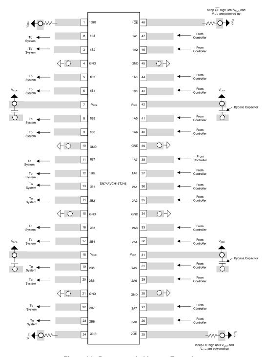
Figure 14. Recommended Layout Example
