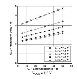
Figure 1. Typical Propagation Delay  $t_{\text{PLH}}$  (A to B) vs Load Capacitance
