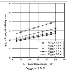
Figure 4. Typical Propagation Delay  $t_{\rm PHL}$  (A to B) vs Load Capacitance
