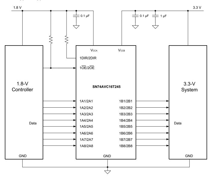
Figure 12. Typical Application Schematic
