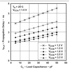
Figure 7-3. Typical Propagation Delay  $t_{\text{PLH}}$  (A to B) vs Load Capacitance
