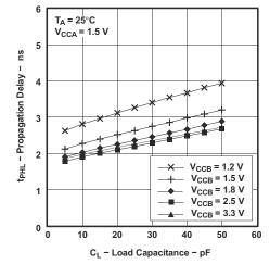
Figure 7-4. Typical Propagation Delay t<sub>PLH</sub> (A to B) vs Load Capacitance
