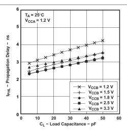
Figure 7-2. Propagation Delay vs Load Capacitance
