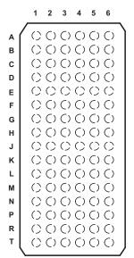
Figure 6-1. GKE, ZKE Package 96-Pin LFBGA Top View
