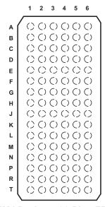
Figure 6-3. NMJ Package 96-Pin nFBGA Top View
