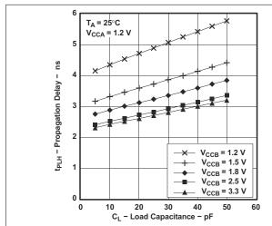
Figure 7-1. Propagation Delay vs Load Capacitance
