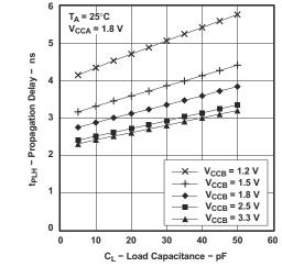
Figure 7-5. Typical Propagation Delay t<sub>PLH</sub> (A to B) vs Load Capacitance
