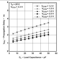
Figure 7-10. Propagation Delay vs Load Capacitance
