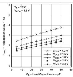
Figure 7-6. Typical Propagation Delay t<sub>PLH</sub> (A to B) vs Load Capacitance
