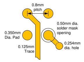
Figure 12-1. BGA Layout Example
