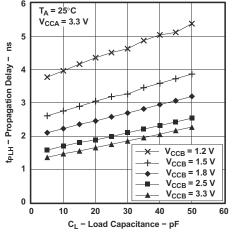
Figure 7-9. Typical Propagation Delay t<sub>PLH</sub> (A to B) vs Load Capacitance
