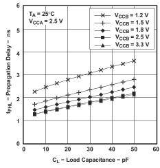
Figure 7-8. Typical Propagation Delay t<sub>PLH</sub> (A to B) vs Load Capacitance
