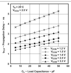
Figure 7-7. Typical Propagation Delay  $t_{\text{PLH}} \ (\text{A to B}) \ \text{vs Load}$  Capacitance
