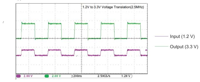
Figure 10-2. Translation Up (1.2 V to 3.3 V) at 2.5 MHz
