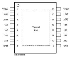
Figure 4-4. DYY Package, 16-Pin SOT (Top View)
