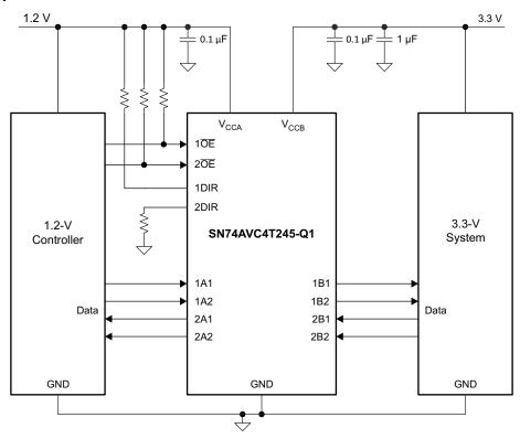
Figure 8-1. Typical Application Diagram
