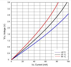
Figure 5-10. Low-Level Output Voltage (V<sub>OL</sub>) vs Low-Level Current (I<sub>OL</sub>)
