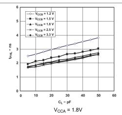
Figure 5-5. Typical Propagation Delay (A to B) vs Load Capacitance
