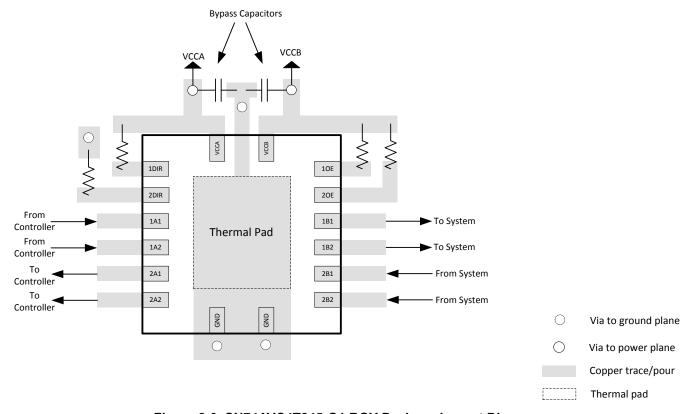
Figure 8-3. SN74AVC4T245-Q1 RGY Package Layout Diagram
