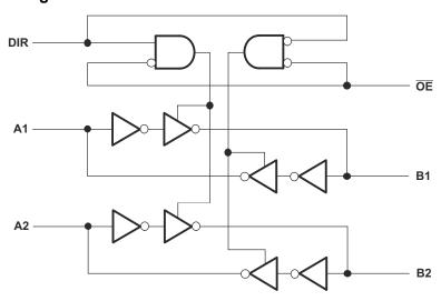
Figure 7-1. Logic Diagram (Positive Logic) for 1/2 of SN74AVC4T245-Q1
