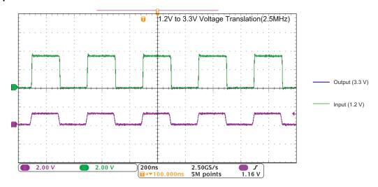
Figure 8-2. Translation Up (1.2V to 3.3V) at 2.5MHz
