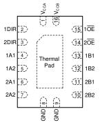
Figure 4-3. BQB/WBQB Package, 16-Pin WQFN (Transparent Top View)
