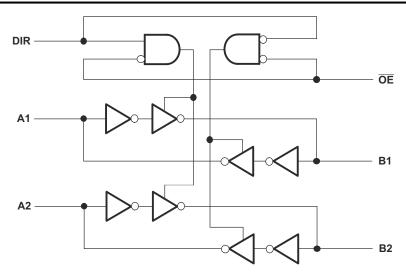
Logic Diagram (Positive Logic) for 1/2 of SN74AVC4T245-Q1
