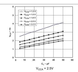
Figure 5-7. Typical Propagation Delay (A to B) vs Load Capacitance
