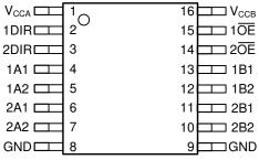
Figure 4-2. PW Package, 16-Pin TSSOP (Top View)
