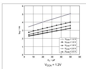
Figure 5-1. Typical Propagation Delay (A to B) vs Load Capacitance
