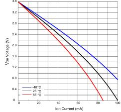
Figure 5-11. High-Level Output Voltage (V<sub>OH</sub>) vs High-Level Current (I<sub>OH</sub>)
