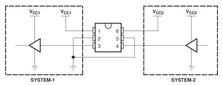
Figure 9-1. Unidirectional Logic Level-Shifting Application Diagram
