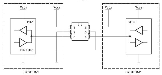
Figure 9-3. Bidirectional Logic Level-Shifting Application Diagram
