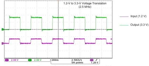
Figure 9-4. Translation Up (1.2V to 3.3V) at 2.5MHz
