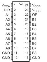
Figure 4-1. DGV or PW Package, 24-Pin TVSOP or TSSOP (Top View)
