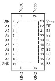
Figure 4-2. RHL Package, 24-Pin VQFN (Top View)
