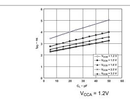
Figure 5-1. Typical Propagation Delay (A to B) vs Load Capacitance
