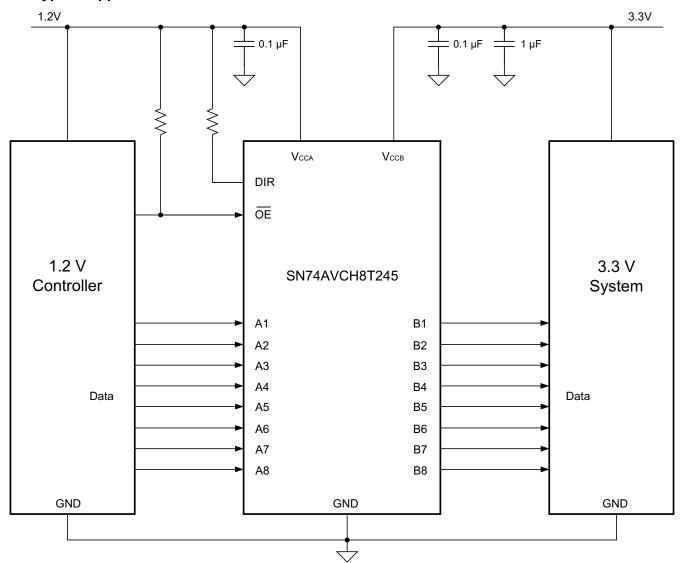
Figure 8-1. Typical Application Schematic
