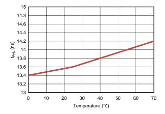
Figure 5. t<sub>PHL</sub> vs Temperature
