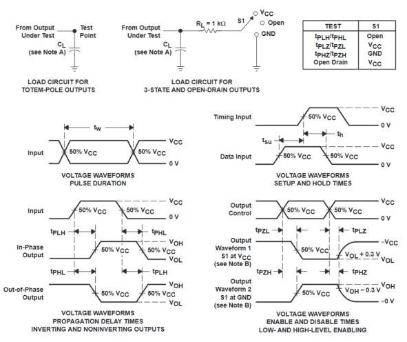
Figure 6-1. Load Circuit and Voltage Waveforms
