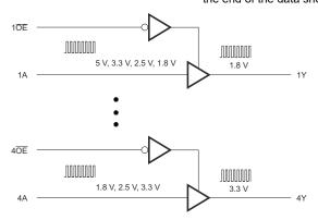
Figure 3-1. Simplified Application Diagram
