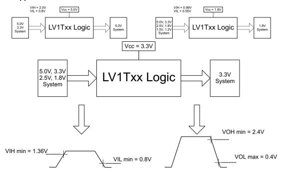
Figure 9-1. Switching Thresholds for 1.8 V to 3.3 V Translation
