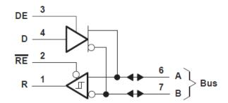
Logic Diagram (Positive Logic)
