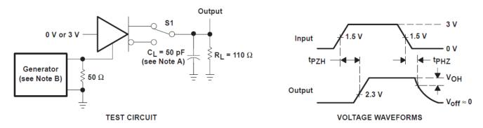
A. C<sub>L</sub> includes probe and jig capacitance.
