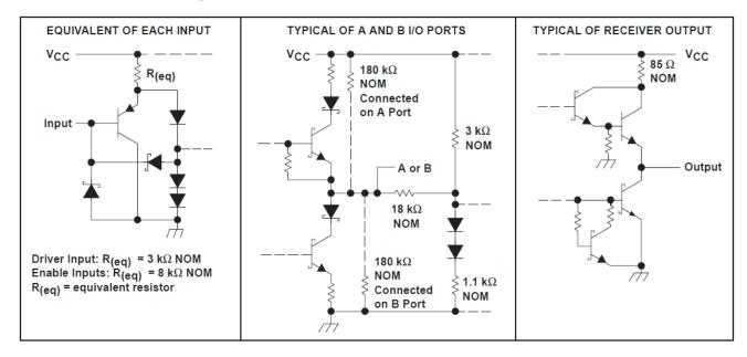
Figure 7-1. Schematic of Inputs and Outputs
