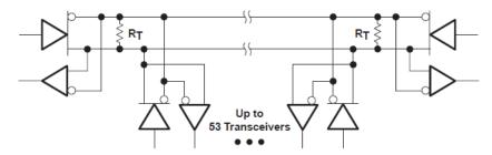
A. The line should terminate at both ends in its characteristic impedance ( $R_T = Z_0$ ). Stub lengths off the main line should be kept as short as possible.
