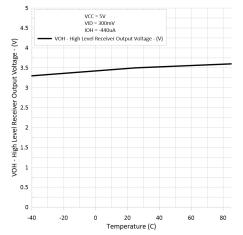
Figure 5-5. Receiver High-Level Output Voltage vs Free-Air Temperature
