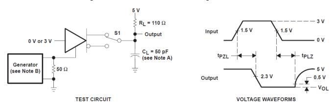
Figure 6-5. Driver Test Circuit and Voltage Waveforms
