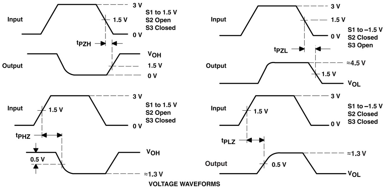
Figure 8. Receiver Output Enable and Disable Times
