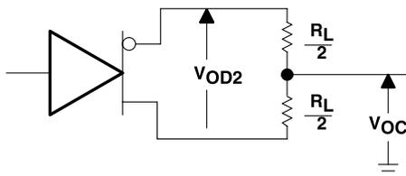
Figure 1. Driver Test Circuit,  $V_{OD}$  and  $V_{OC}$
