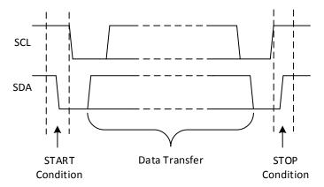
Figure 8-3. Definition of Start and Stop Conditions
