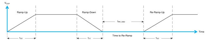
Figure 9-6.  $V_{CCP}$  is Lowered Below 0.2 V and then Ramped Up to  $V_{CCP}$
