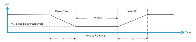
Figure 9-7. V<sub>CCP</sub> is Lowered Below the POR Threshold, then Ramped Back Up to V<sub>CCP</sub>
