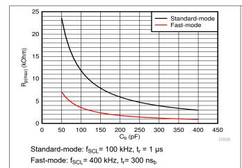
Figure 9-4. Maximum Pull-Up Resistance  $(R_{p(max)})$  vs Bus Capacitance (C)
