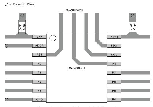
Figure 9-10. Example Layout (PW Package)
