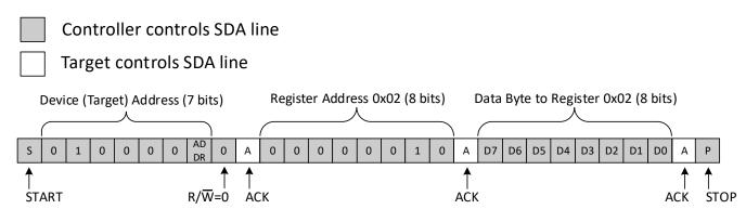
Figure 8-6. Write to the Polarity Inversion Register
