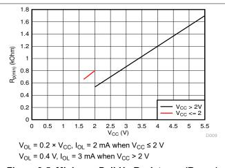
Figure 9-5. Minimum Pull-Up Resistance ( $R_{p(min)}$ ) vs Pull-Up Reference Voltage ( $V_{CCI}$ )
