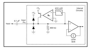
Figure 100. Equivalent AC Sync-Tip-Clamp Input
