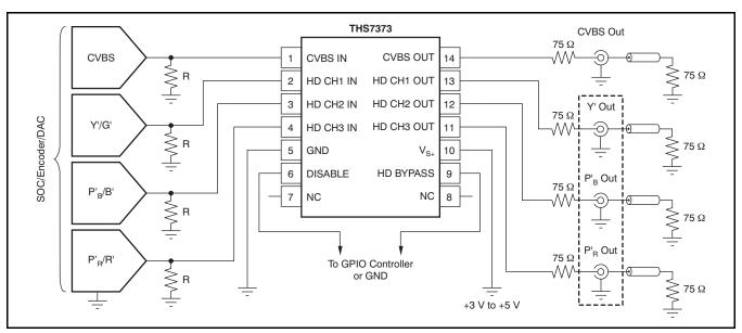
Figure 98. Typical Four-Channel System Inputs from DC-Coupled Encoder/DAC with DC-Coupled Line Driving
