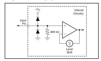
Figure 99. Equivalent DC Input Mode Circuit
