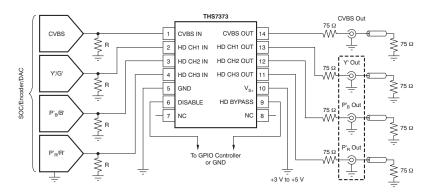
Figure 1. Single-Supply, DC-Input/DC-Output Coupled Video Line Driver
