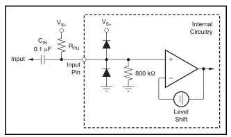
Figure 101. AC-Bias Input Mode Circuit Configuration
