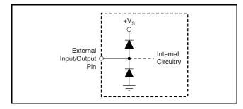
Figure 97. Internal ESD Protection
