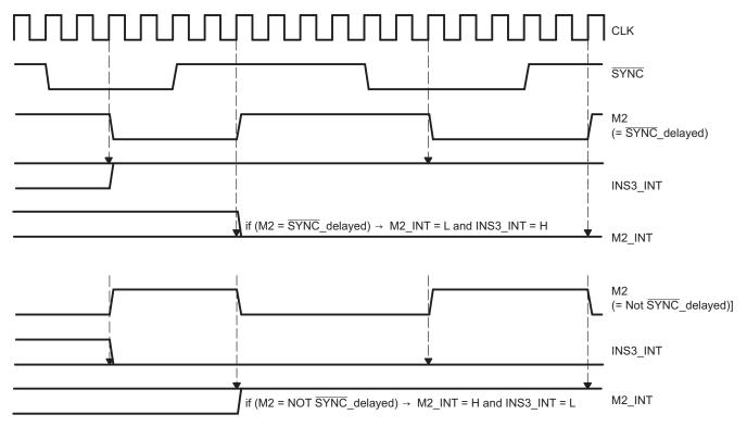
Figure 6. Generating INS3\_INT and M2\_INT From M2
