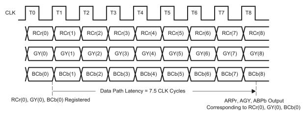
Figure 7. Input Format and Latency YCbCr 4:4:4 and GBR 4:4:4 Modes
