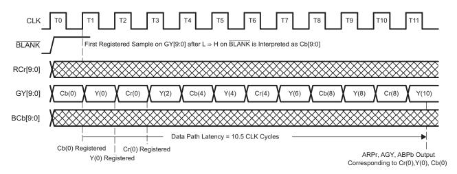
Figure 9. Input Format and Latency YCbCr 4:2:2 1x10-Bit Mode
