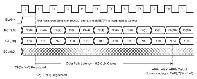
Figure 8. Input Format and Latency YCbCr 4:2:2 2x10-Bit Mode
