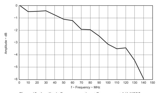
Figure 15. Amplitude Response vs Input Frequency at 240 MSPS
