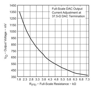
Figure 5. Output Voltage vs Full-Scale Resistance
