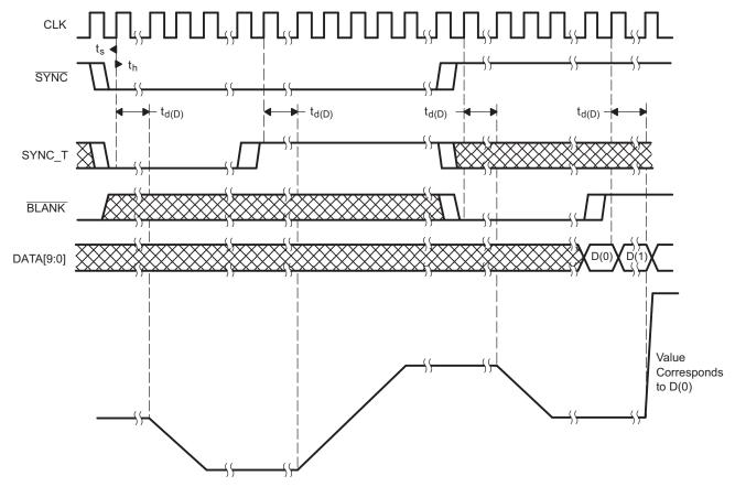
Figure 10. Sync and Blanking Generation
