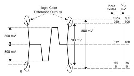
Figure 4. CbCr Outputs, Reduced-Scale Input Code Range
