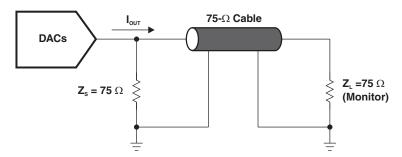
Figure 2. DAC Output Termination
