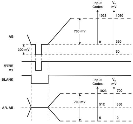
NOTE:  $R_{FS}$  chosen for 700-mV output.
