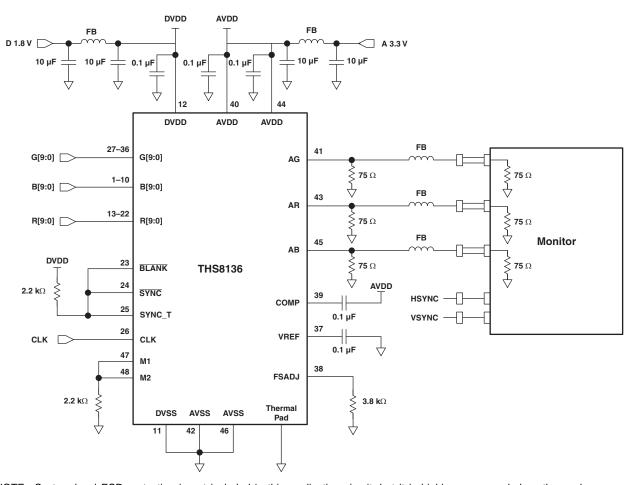
NOTE: System level ESD protection is not included in this application circuit, but it is highly recommended on the analog RGB outputs.
