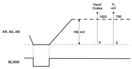
NOTE: BLANK = High in applications not requiring a forced blank level.
