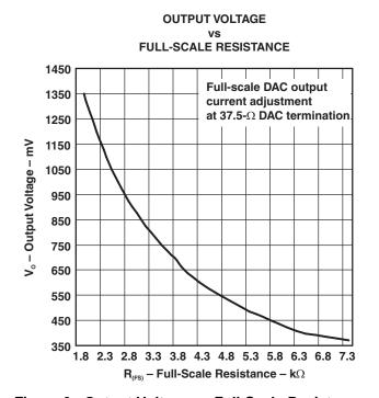
Figure 3. Output Voltage vs Full-Scale Resistance
