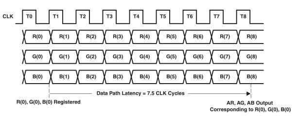
Figure 7. Input Data Internally Latched on Rising Edge of CLK (Data Path Latency is 7.5 CLK Cycles)
