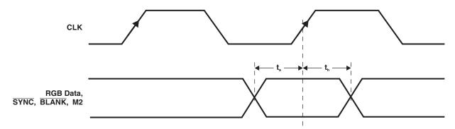
Figure 8. Input Data Registered on Rising Edge of CLK
