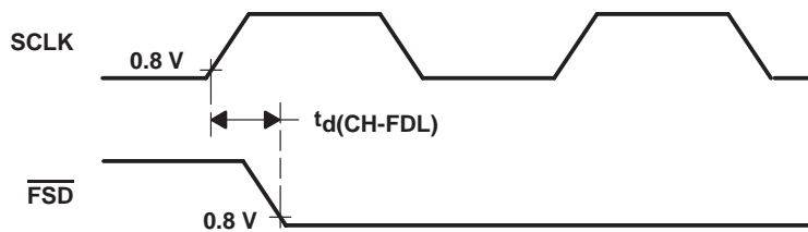
Figure 5–2. Slave \overline{\text{FS}} to \overline{\text{FSD}} Timing
