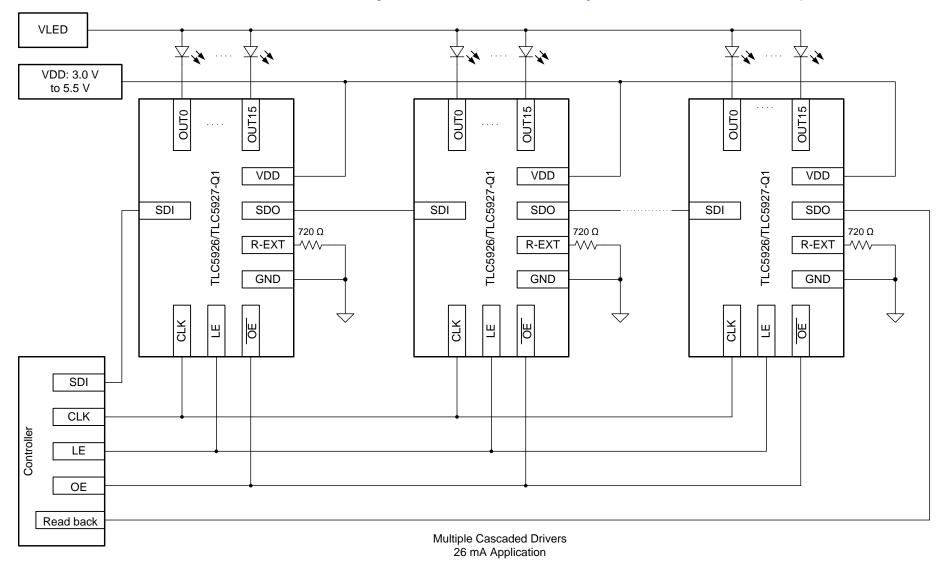
Figure 20. Cascading Implementation of TLC592x-Q1 Schematic
