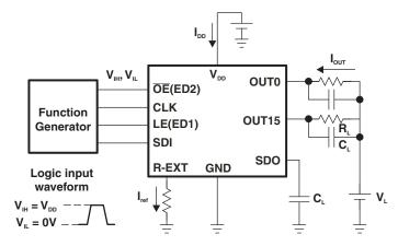
Figure 3. Test Circuit for Switching Characteristics
