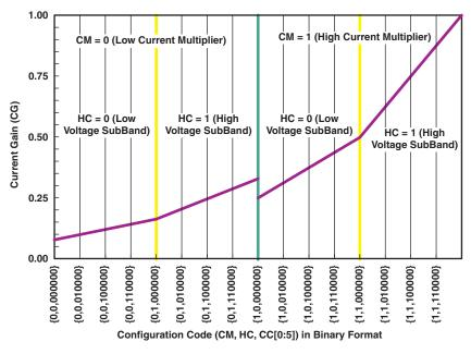
Figure 17. Current Gain vs Configuration Code
