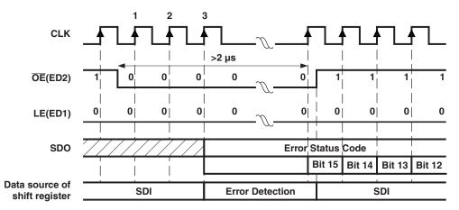
Figure 14. Reading Error Status Code
