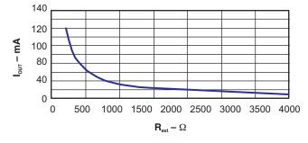
Figure 16. Default Relationship Curve Between I<sub>OUT,target</sub> and R<sub>ext</sub>
