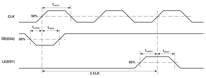
Figure 5. Switching to Special Mode Timing Waveforms
