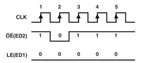
Figure 12. Switching to Normal Mode
