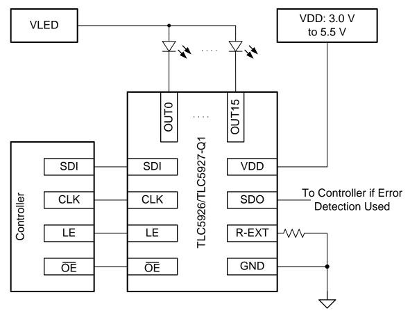
Figure 18. Simple Implementation of TLC591x-Q1 Circuit
