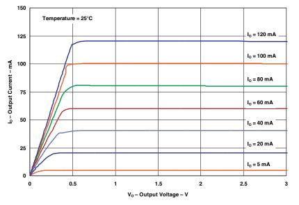
Figure 19. Output Current vs Output Voltage
