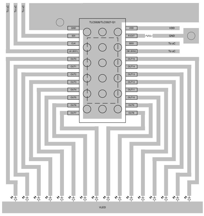
Figure 21. TLC592x-Q1 Layout Example
