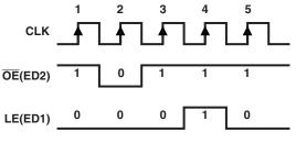
Figure 9. Switching to Special Mode
