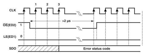
Figure 11. Reading Error Status Code
