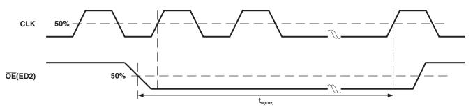
Figure 6. Reading Error Status Code Timing Waveforms
