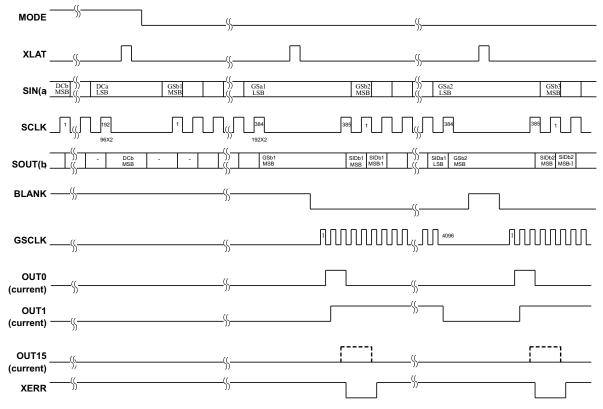
Figure 14. Timing Chart for Two Cascaded TLC5941-Q1 Devices
