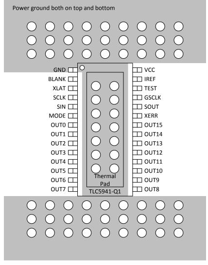
Figure 25. PCB Layout Example
