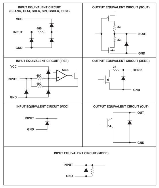
Figure 10. Input and Output Equivalent Circuits
