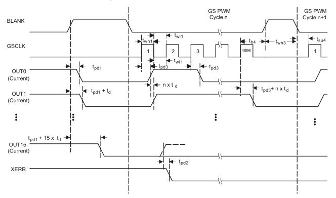
Figure 17. Grayscale PWM Cycle Timing Chart
