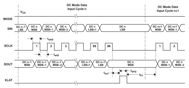
Figure 20. Dot-Correction Data Input-Timing Chart
