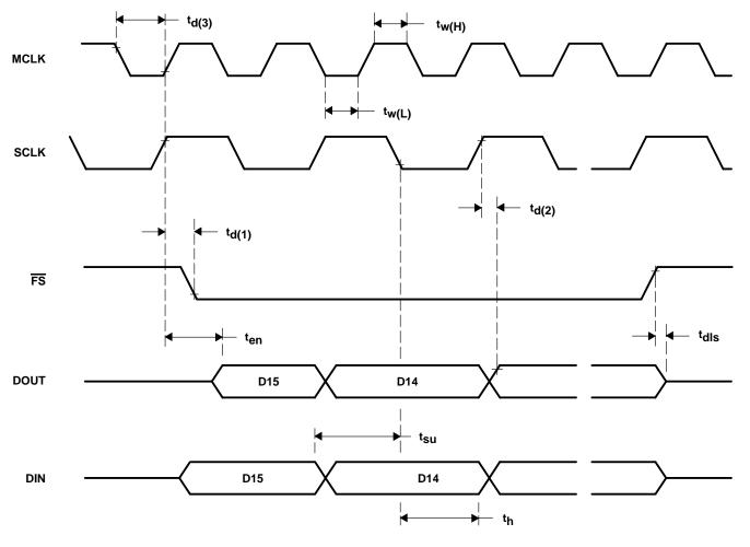
Figure 5–2. Serial Communication Timing
