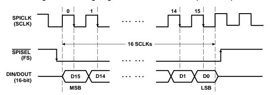
Figure 2-9. Timing Diagram for the SPI\_CP0 Mode (M1M0 = 01)
