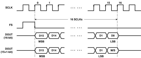
NOTES: A. M/S is used to indicate whether the 15-bit data comes from a master or a slave device (master: M/S=1, slave: M/S=0).
