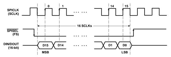
Figure 2–10. Timing Diagram for the SPI\_CP1 Mode (M1M0 = 10)
