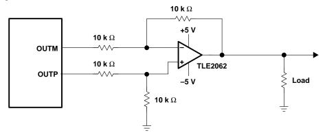
Figure 2–17. Differential Output Drive (Ground-Referenced)
