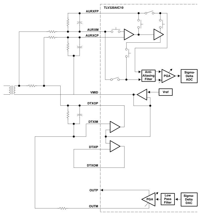
Figure A-2. Single-Ended Configuration of Hybrid Connection
