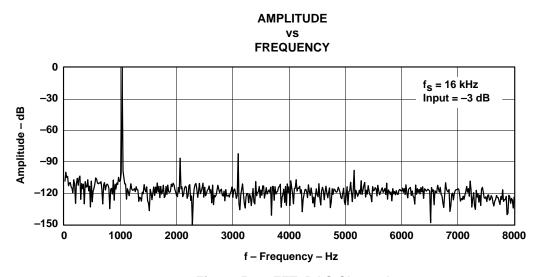
Figure 5-6. FFT-DAC Channel
