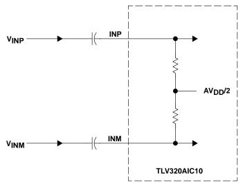
Figure 2–16. INP and INM Internal Self-Biased (AV<sub>DD</sub>/2) Circuit
