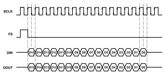
Figure 3–1. Primary Serial Communication Timing
