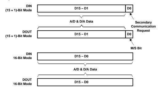
Figure 3-11. Primary Communication DIN and DOUT Data Format
