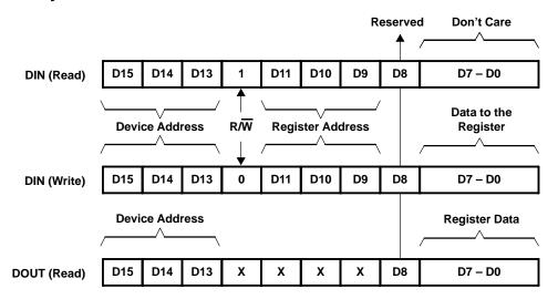
Figure 3-12. Secondary Communication DIN and DOUT Data Format
