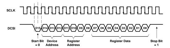
Figure 3-9. Direct Configuration Mode Timing
