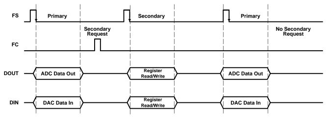
Figure 3–5. FS Output When Hardware Secondary Serial Communication Is Requested Only Once (No Slave)
