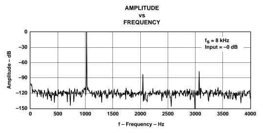
Figure 5-9. FFT-DAC Channel
