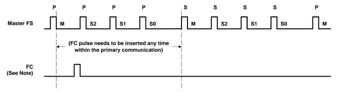
NOTES: A. FC of master device and slave devices should be connected together
