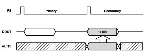
NOTE A: When DIN performs a write operation (sets D12 to 0) during secondary communication.
