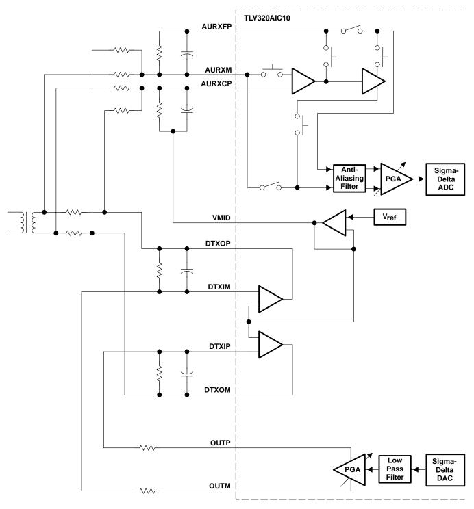
Figure A-1. Differential Configuration for Hybrid Connection
