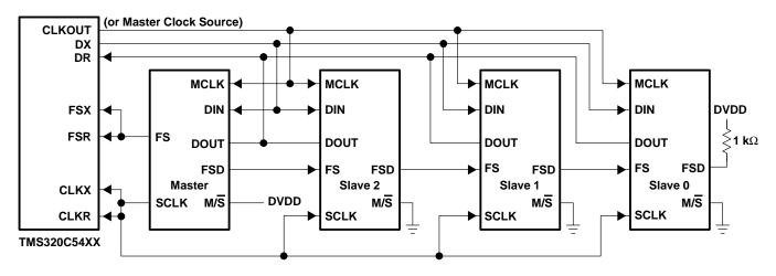
Figure 2–14. Cascade Mode Connection (to DSP Interface)
