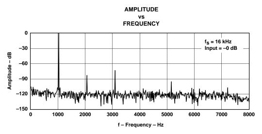
Figure 5-10. FFT-DAC Channel
