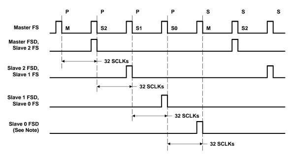
Figure 2-15. Master-Slave Frame-Sync Timing
