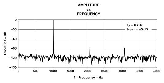
Figure 5-5. FFT-DAC Channel
