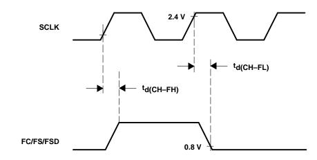
Figure 5-1. FC, FS, and FSD Timing
