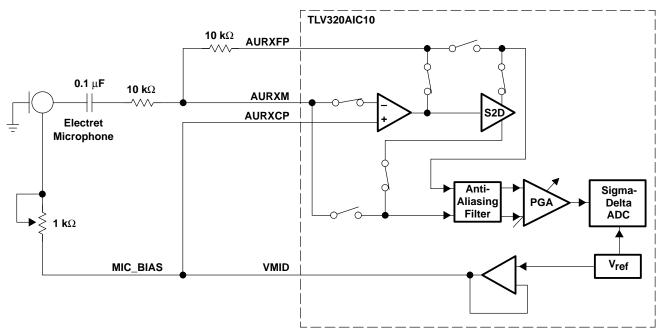
Figure 2-5. Typical Microphone Interface
