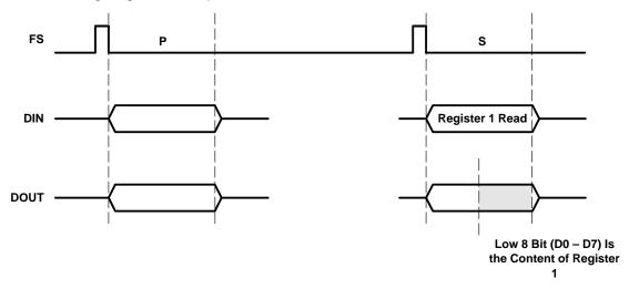
Figure 3–3. Device 3/Register 1 Read Operation Timing Diagram
