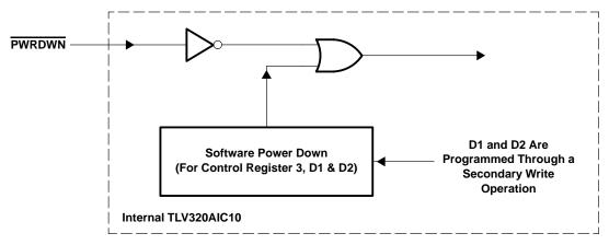
Figure 2–7. Internal Power-Down Logic
