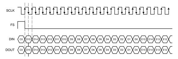
Figure 3–10. Continuous Data Transfer Mode Timing
