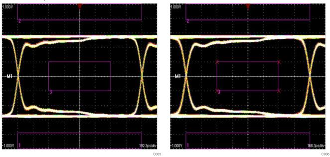
Figure 31. TMDS Data Rate of 650 Mbps
