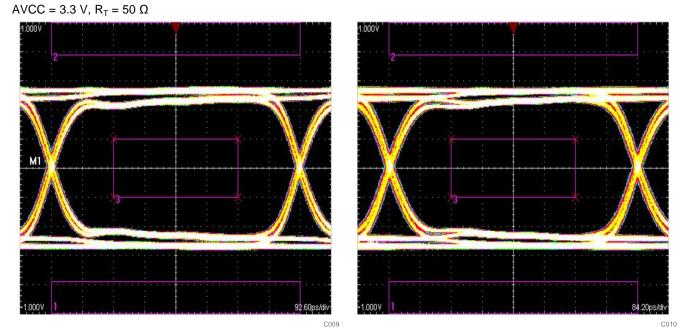
Figure 35. TMDS Data Rate of 1350 Mbps
