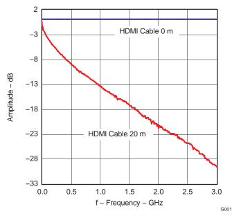
Figure 15. Loss Profile of 20-m HDMI Cable
