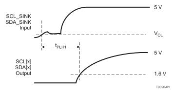
Figure 8. Source-Side Output AC Measurements (Continued)
