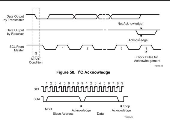
Figure 51. I<sup>2</sup>C Address, Data Cycle(s), and Stop
