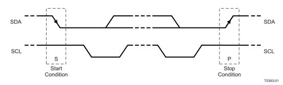
Figure 48. I<sup>2</sup>C Start and Stop Conditions
