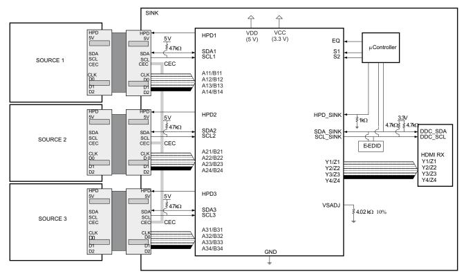
Figure 46. Three-Port HDMI-Enabled DTV With TMDS361B – CEC Commands Passing Through
