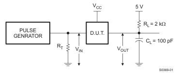
Figure 4. Sink-Side Test Circuit
