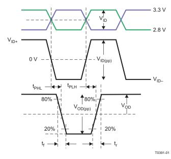
Figure 10. TMDS Main-Link Timing Measurements
