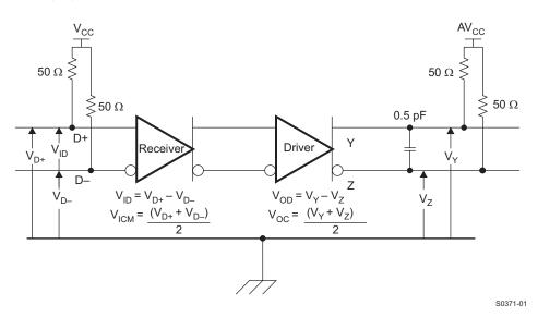
Figure 9. TMDS Main-Link Test Circuit
