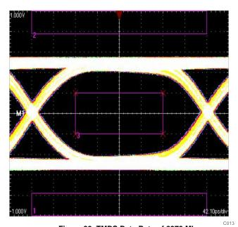
Figure 39. TMDS Data Rate of 2970 Mbps
