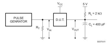
Figure 5. Source-Side Test Circuit
