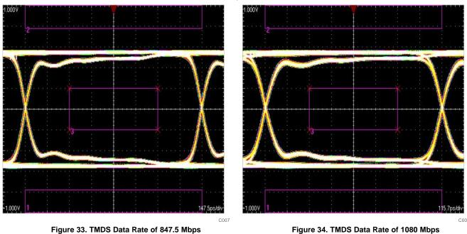
Figure 34. TMDS Data Rate of 1080 Mbps
