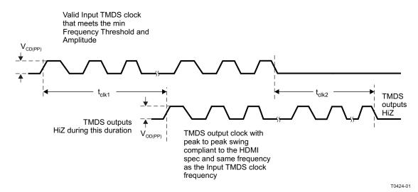
Figure 13. Clock-Detect Timing Diagram
