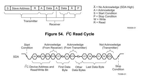
Figure 55. Multiple-Byte Read Transfer
