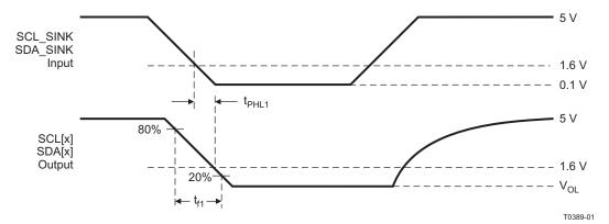
Figure 7. Sink-Side Output AC Measurements
