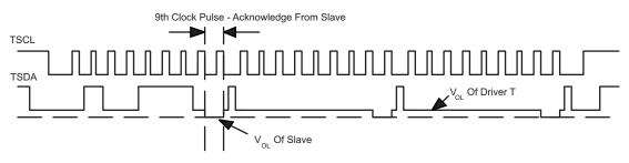
Figure 44. Bus-T Waveform
