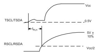
Figure 41. Waveform of Driver T Turning Off
