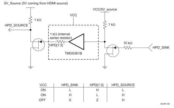
Figure 45. External Circuit to Drive 5-V V<sub>OH</sub> on HPD[1:3]
