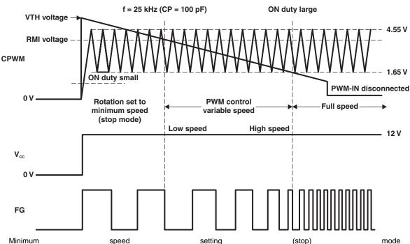
A. Minimum speed setting (stop) mode PWM-IN input is filtered to generate the VTH voltage. At low speed, the fan rotates with the minimum speed set with RMI during low speed. If the minimum speed is not set (RMI = 6VREG), the fan stops.
