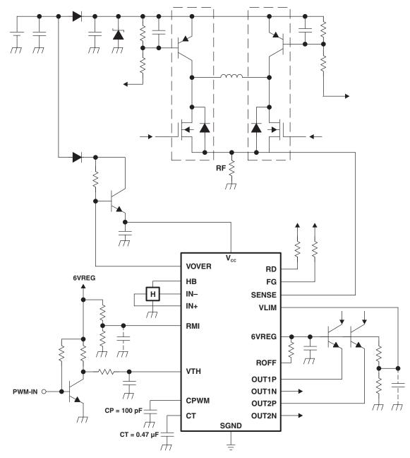
Figure 7. 24-V/48-V Sample Application Circuit
