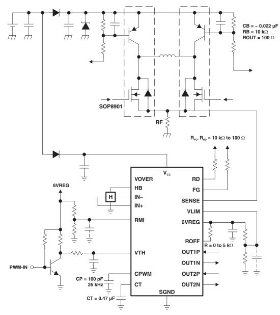
Figure 3. 12-V Sample Application Circuit
