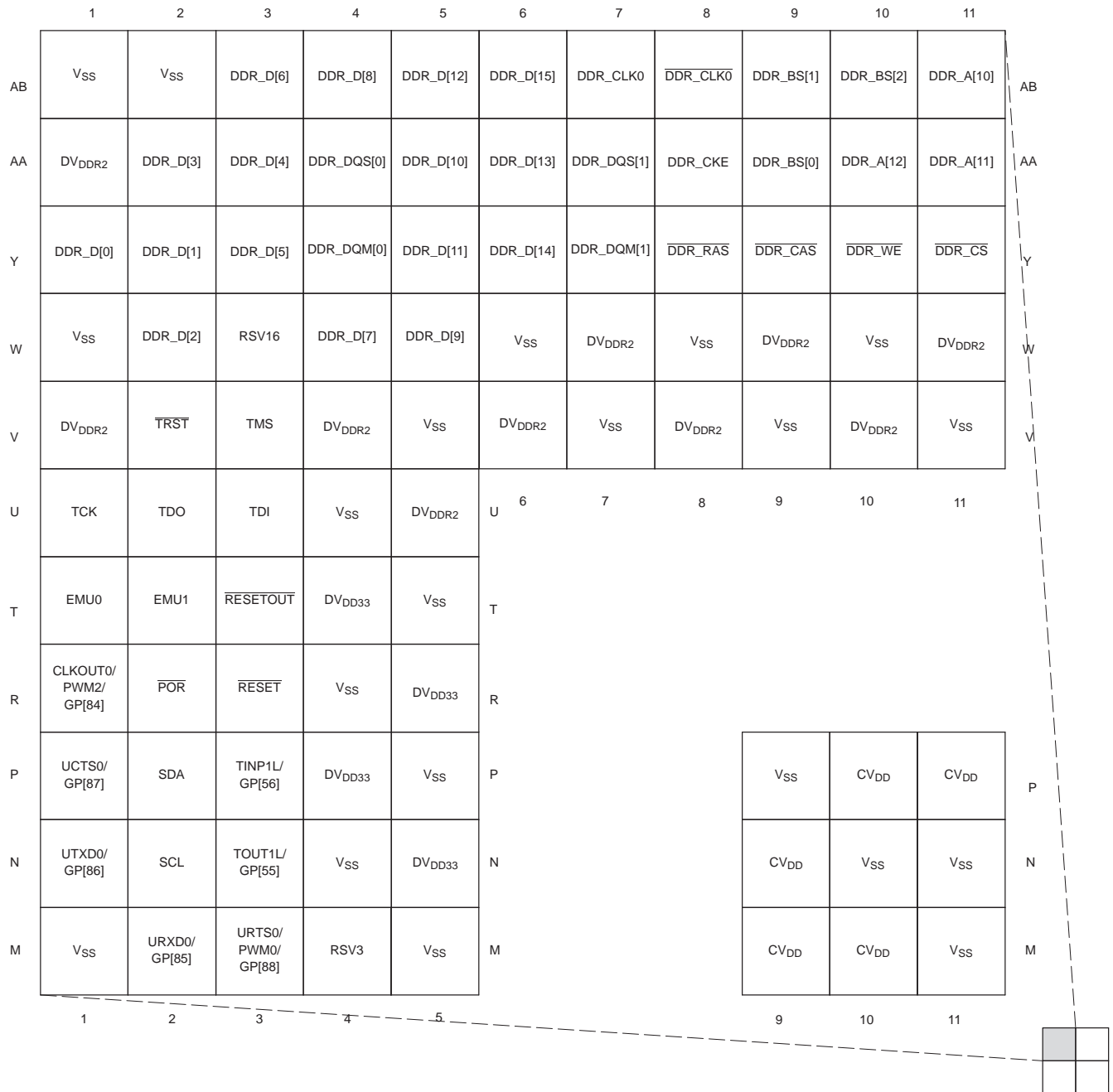
Figure 2-8. ZDU Pin Map [Quadrant A]
